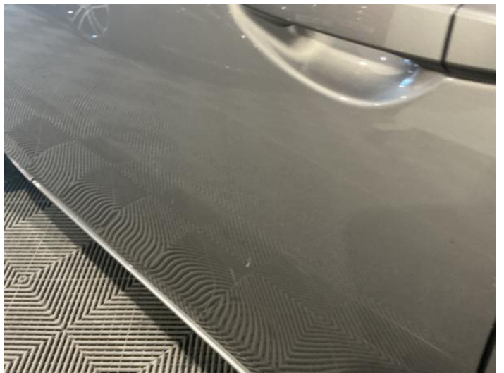
6: Door nsf Scratched Over 25mm Thru Paint
