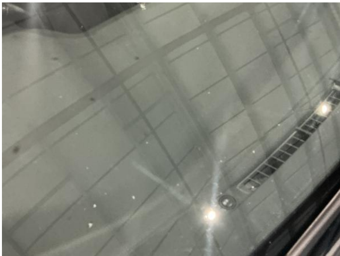
21: Screen Front Chipped UpTo 10mm
