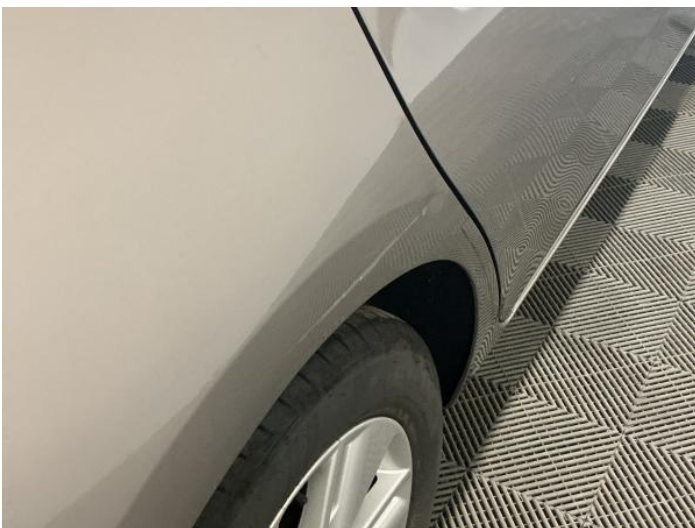
13: Qtr Panel osr Dented With Paint Damage
