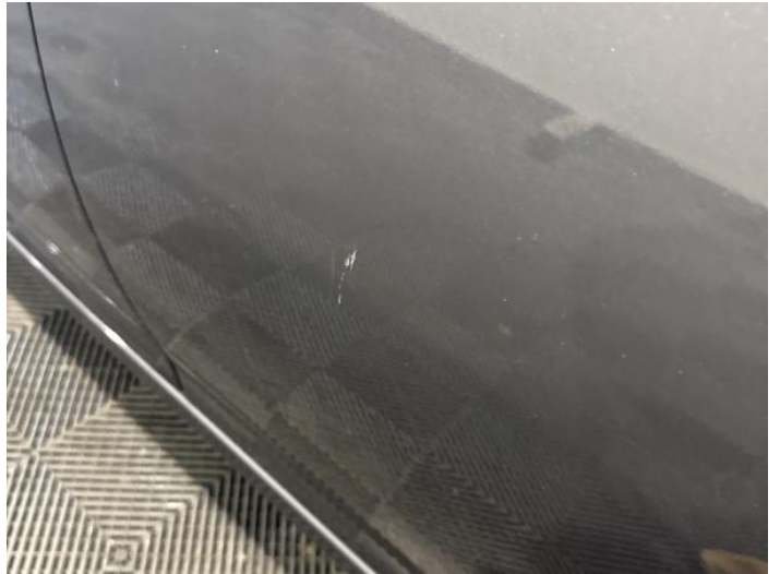
10: Door nsr Scratched Over 25mm Thru Paint
