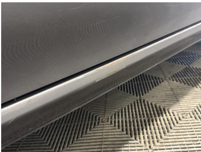
17: Sill os Scratched Rusted
