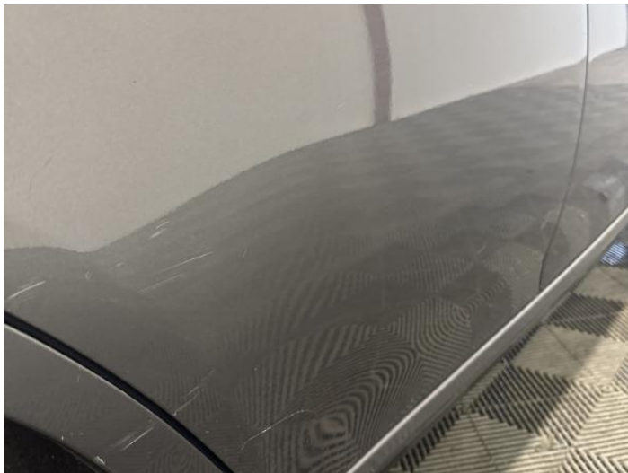
15: Door osr Scratched Over 25mm Thru Paint
