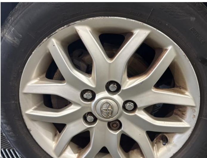
7: Wheel nsf Scratched Over 50mm
