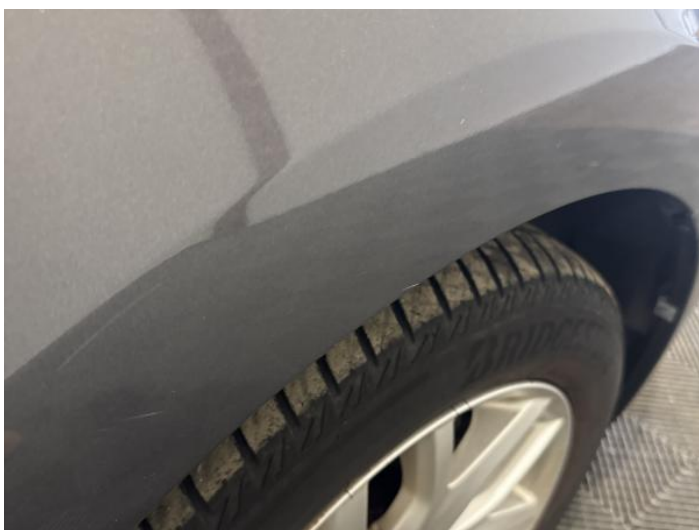
19: Wing osf Scratched UpTo 25mm Thru Paint
