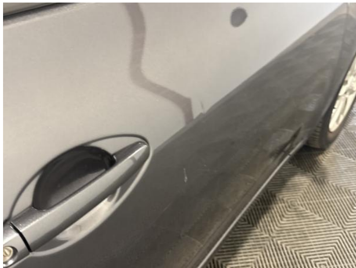
16: Door osf Dented Over 30mm
