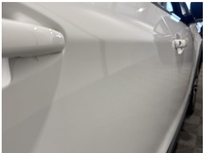
8: Door osr Poor Previous Repair Rippled UpTo 30%
