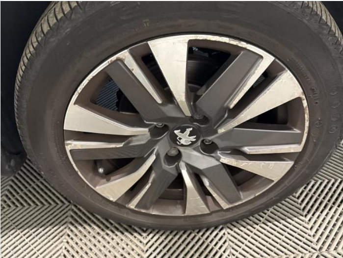
10: Wheel osf Scratched Over 50mm
