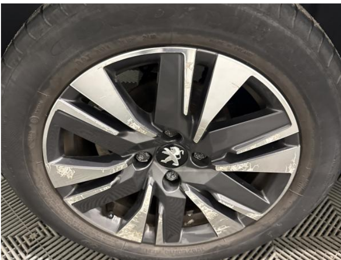
7: Wheel osr Corroded Light
