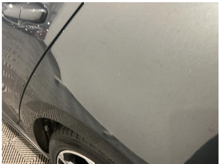
8: Qtr Panel nsr Dented Over 2 UpTo 10mm
