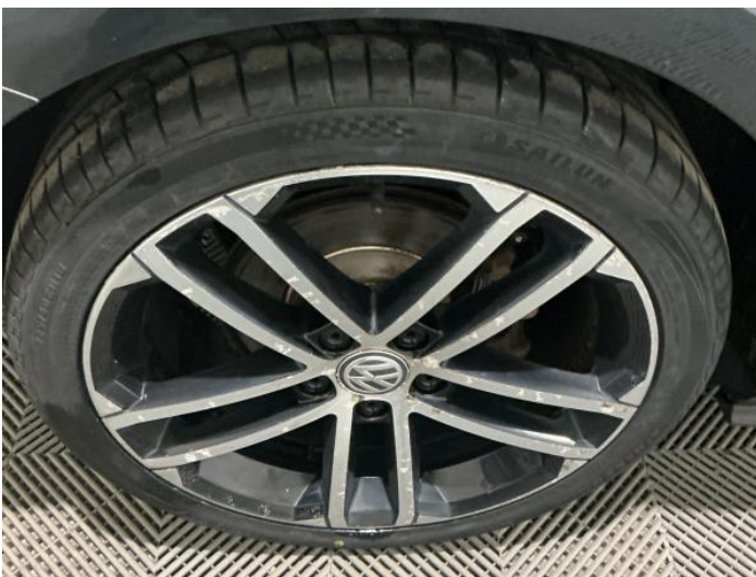
13: Wheel osr Scratched Over 50mm
