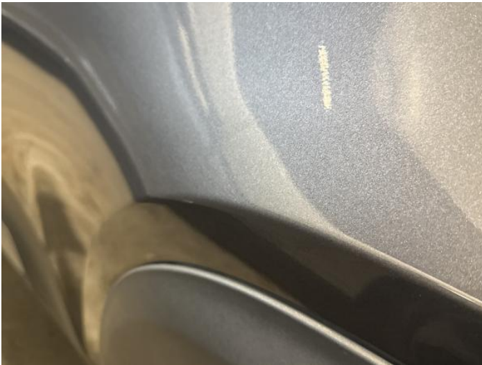
5: Door nsr Scratched UpTo 25mm Thru Paint
