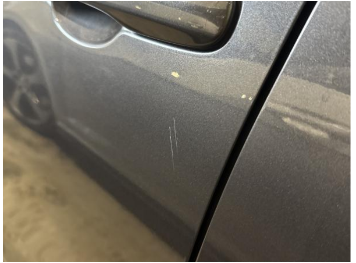
4: Door nsf Scratched UpTo 25mm Thru Paint
