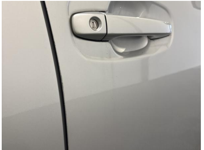
12: Door osf Chipped Edge Chip
