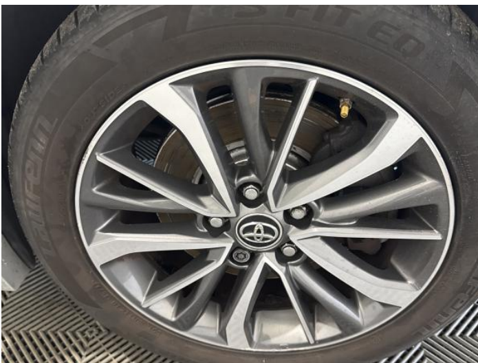
13: Wheel osf Scratched Over 50mm
