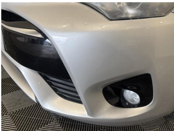
1: Bumper Front Scratched Over 100mm Thru Paint
