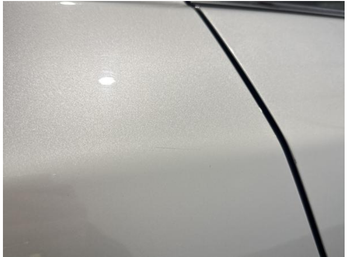
10: Qtr Panel osr Scratched UpTo 25mm Thru Paint
