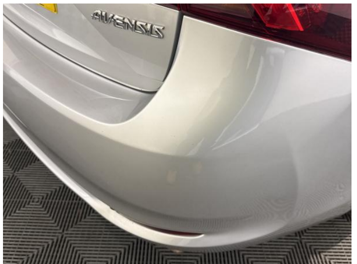
8: Bumper Rear Scratched 25 to 100mm Thru Paint
