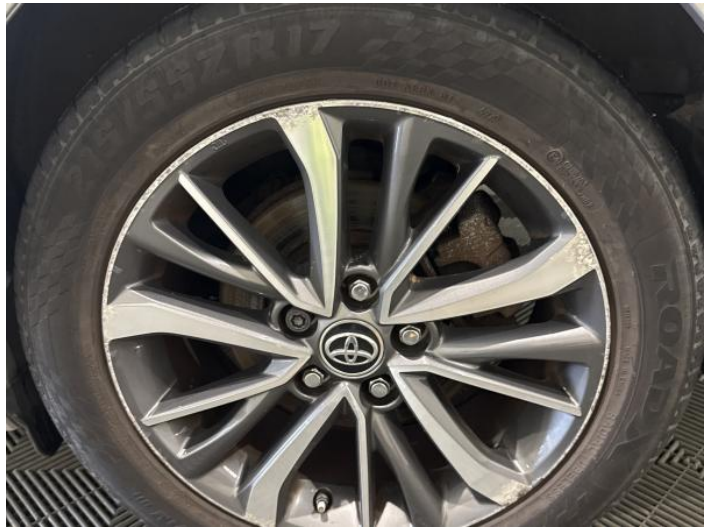
6: Wheel nsr Scratched Over 50mm
