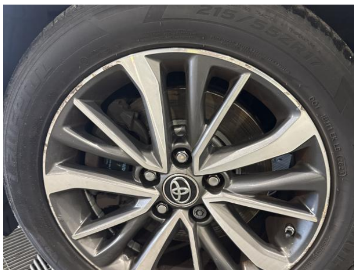
2: Wheel nsf Scratched Over 50mm
