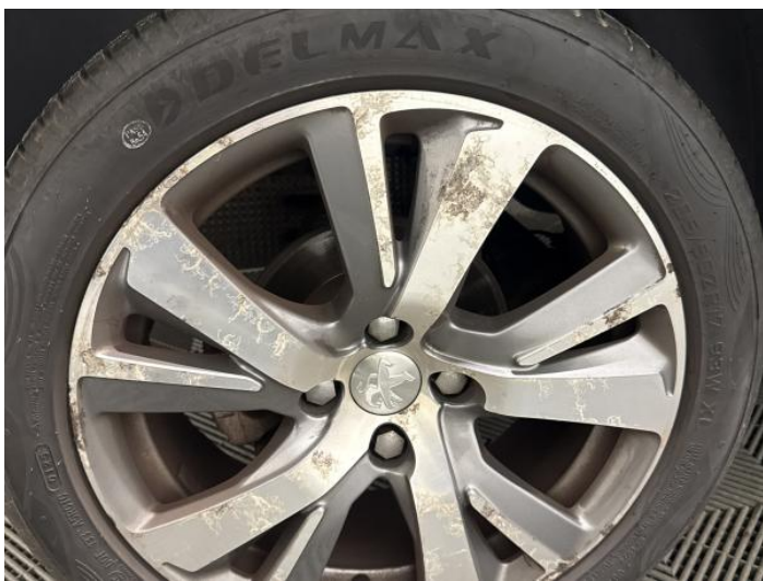
11: Wheel osr Scratched Over 50mm
