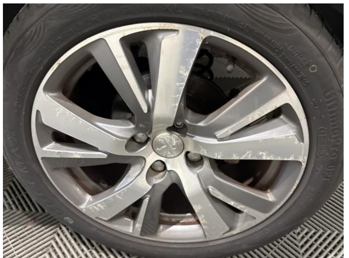
8: Wheel nsr Corroded Light
