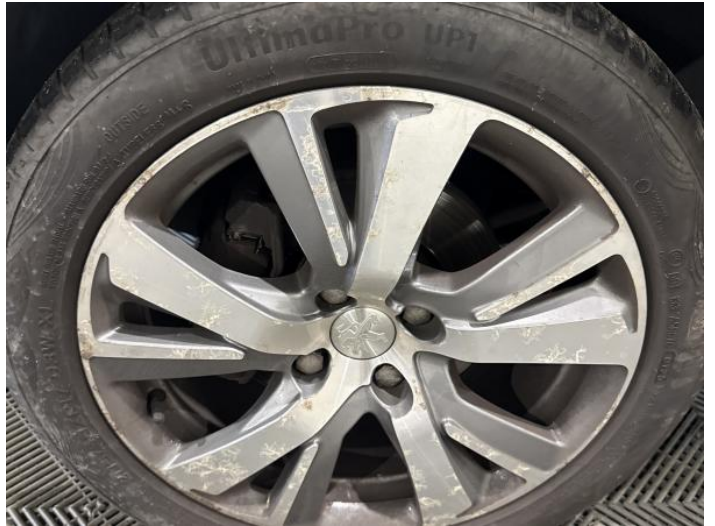
4: Wheel nsf Scratched Over 50mm
