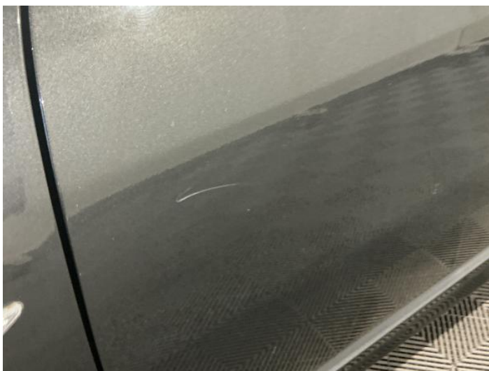
5: Door nsf Scratched Over 25mm Thru Paint
