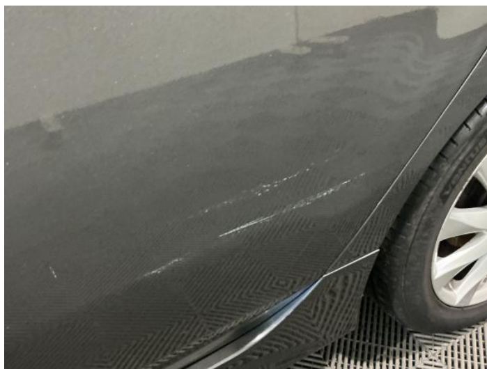
6: Door nsr Scratched Over 25mm Thru Paint
