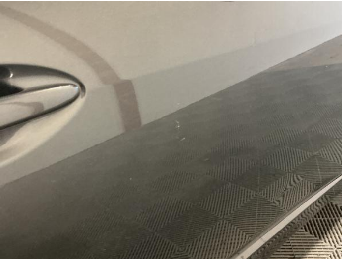
17: Door osf Chipped Multiple Chips
