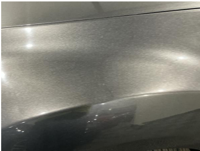
3: Wing nsf Dented Over 30mm
