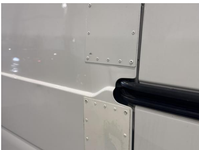
7: Door nsr Hole Over 10mm
