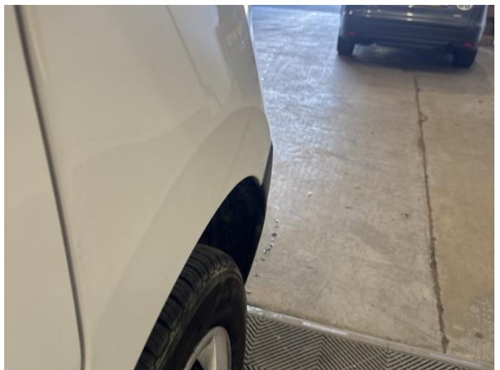
14: Wing osf Dented Over 30mm
