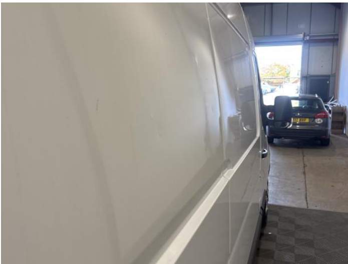
11: Qtr Panel osr Dented Over 30mm
