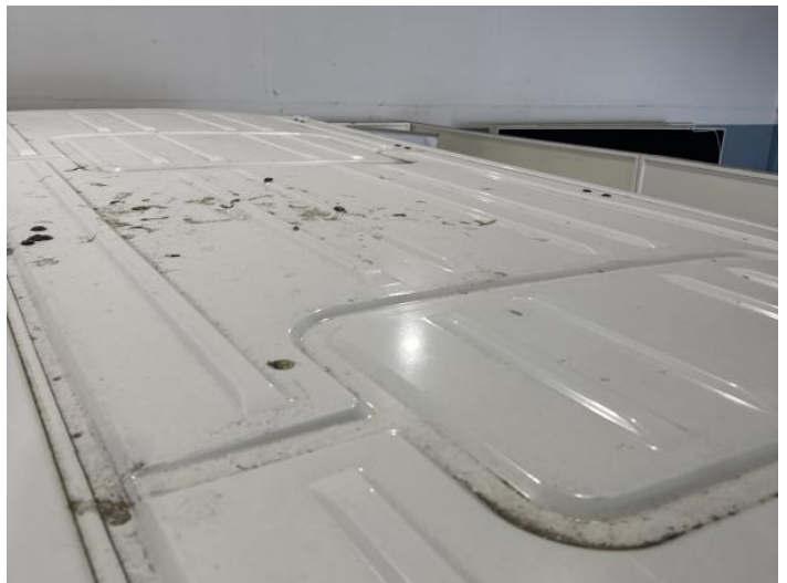
16: Roof Dented Over 30mm
