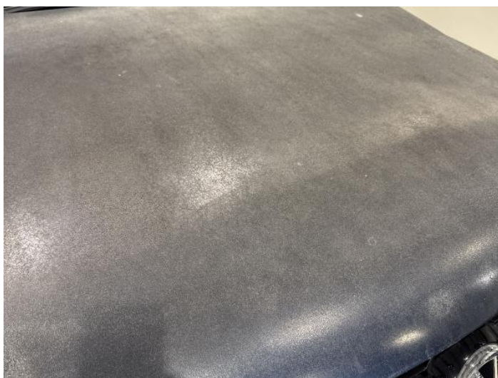
1: Bonnet Poor Previous Repair Poor Paint
