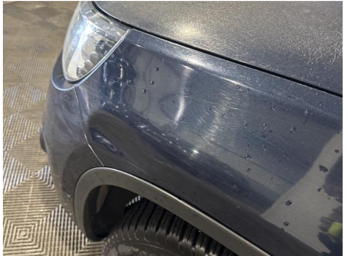
4: Wing nsf Dented With Paint Damage
