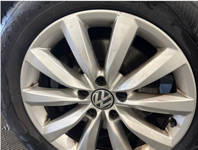
5: Wheel nsf Scratched Up To 50mm
