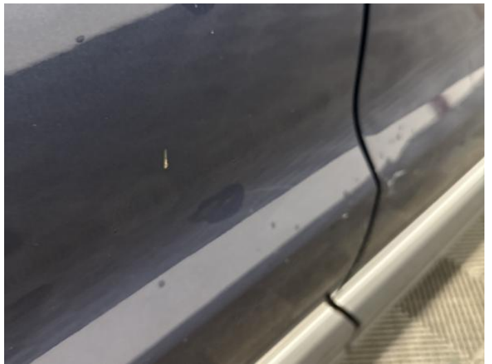
12: Door osr Scratched Over 25mm Thru Paint
