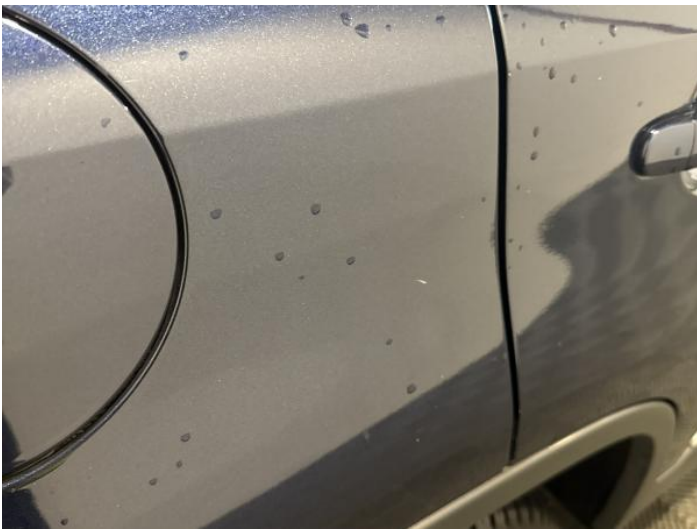
11: Qtr Panel osr Scratched UpTo 25mm Thru Paint
