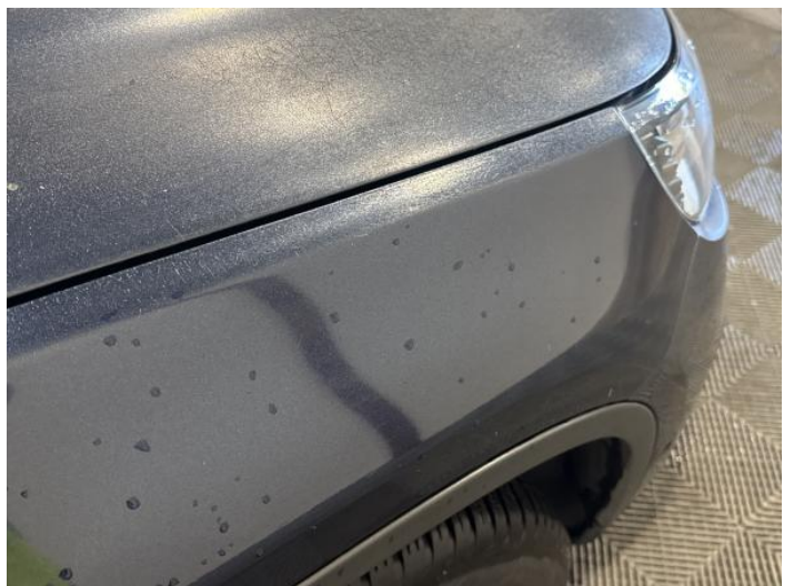
14: Wing osf Poor Previous Repair Poor Paint
