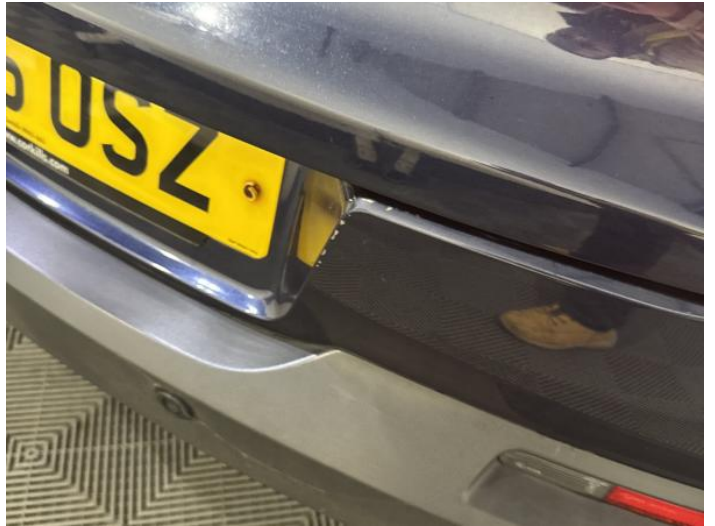
10: Bumper Front Scratched 25 to 100mm Thru Paint
