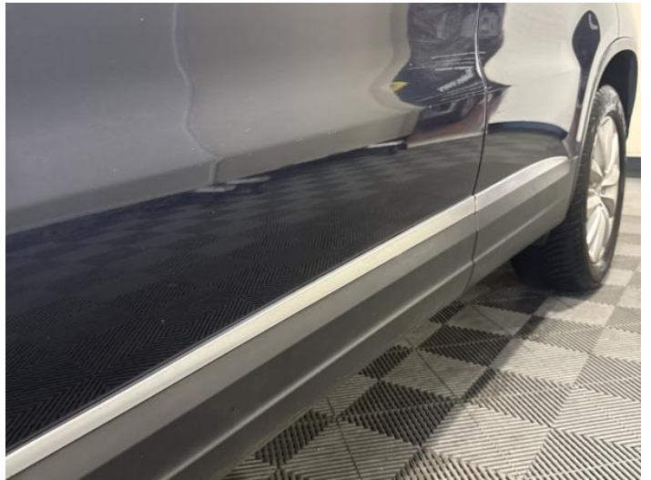
6: Door nsf Dented Between 10mm + 30mm
