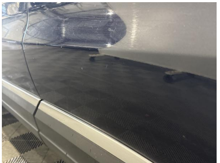
8: Door nsr Scratched Over 25mm Thru Paint
