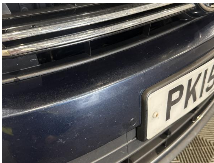
2: Bumper Front Poor Previous Repair Poor Paint
