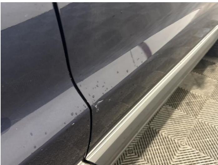
13: Door osf Dented With Paint Damage
