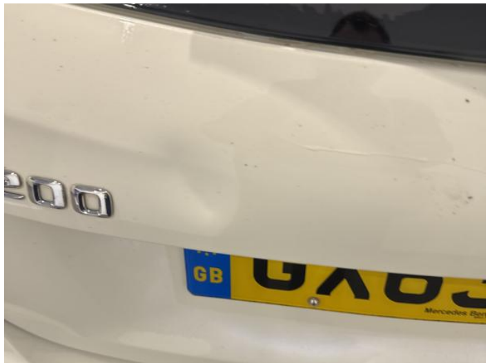
16: Boot Lid Dented Over 30mm
