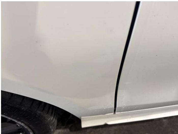
5: Wing nsf Dented Over 30mm
