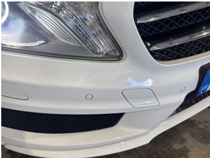
3: Bumper Front Chipped Multiple Chips
