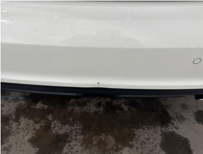
9: Bumper Rear Dented Over 30mm
