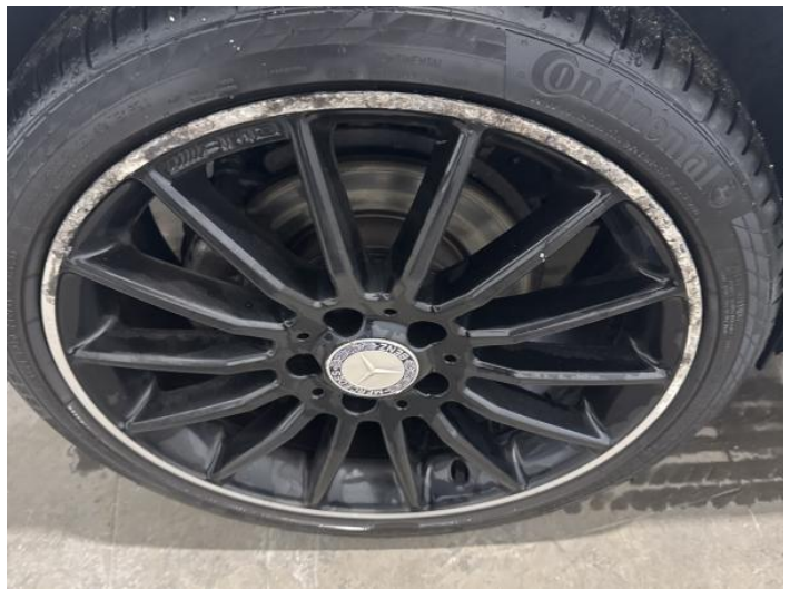
12: Wheel osr Scratched Over 50mm
