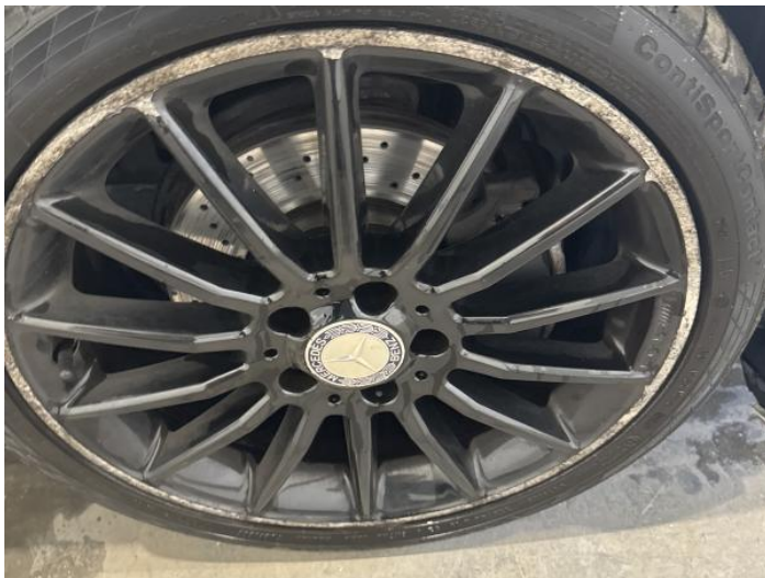
15: Wheel osf Scratched Over 50mm
