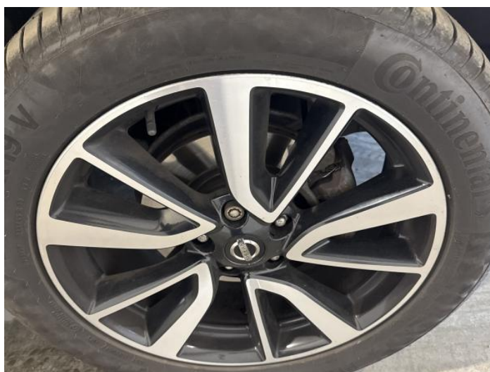
12: Wheel osf Scratched Up To 50mm
