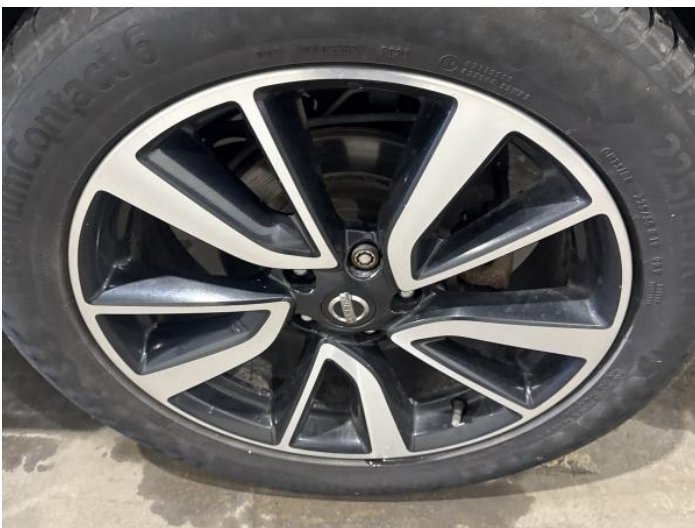
7: Wheel nsr Scratched Up To 50mm
