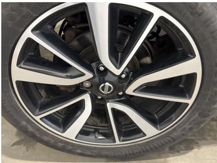
9: Wheel osr Scratched Up To 50mm
