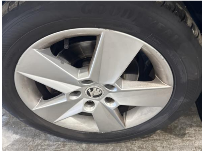
4: Wheel nsf Scratched Over 50mm
