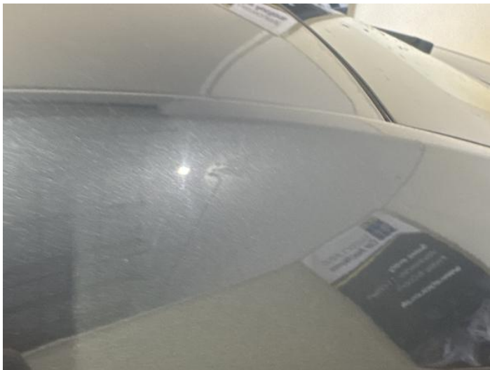
15: D Post ns Dented Over 2 UpTo 10mm
