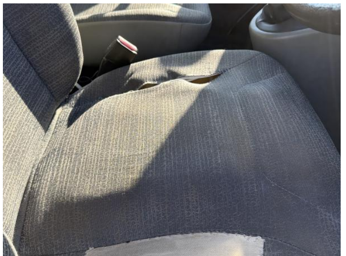
14: Seat Base Cover osf Torn Over 3mm
