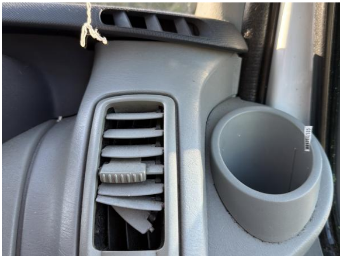
15: Air Vents of Damaged Replace
