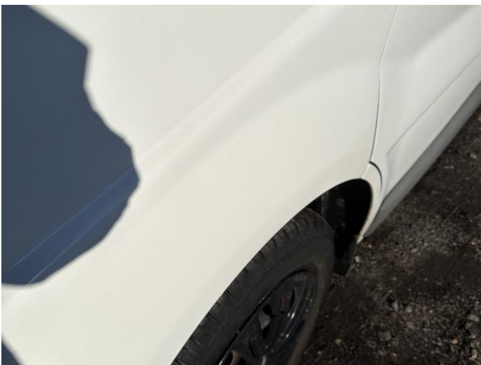
7: Wing nsf Dented Over 2 UpTo 10mm
