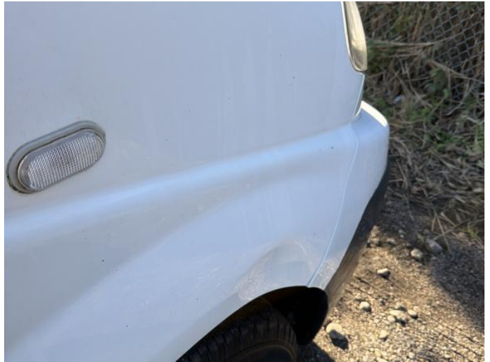
4: Wing osf Dented With Paint Damage
