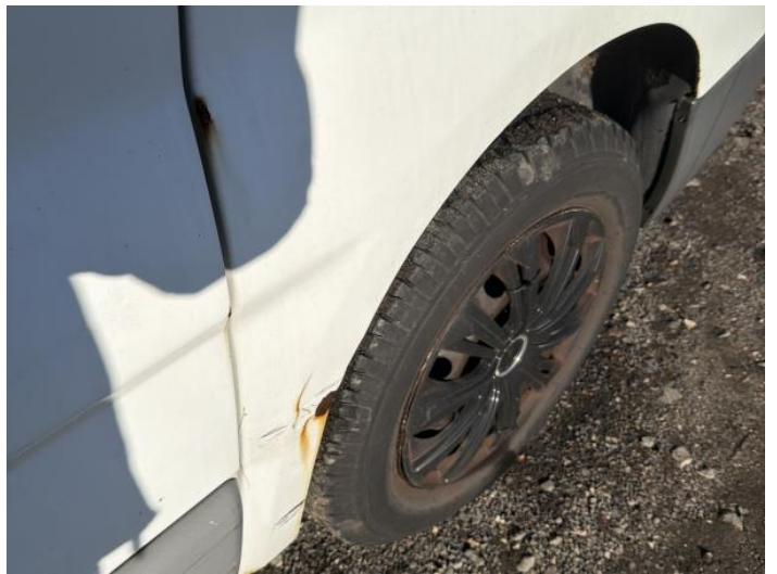
12: Qtr Panel nsr Dented With Paint Damage
