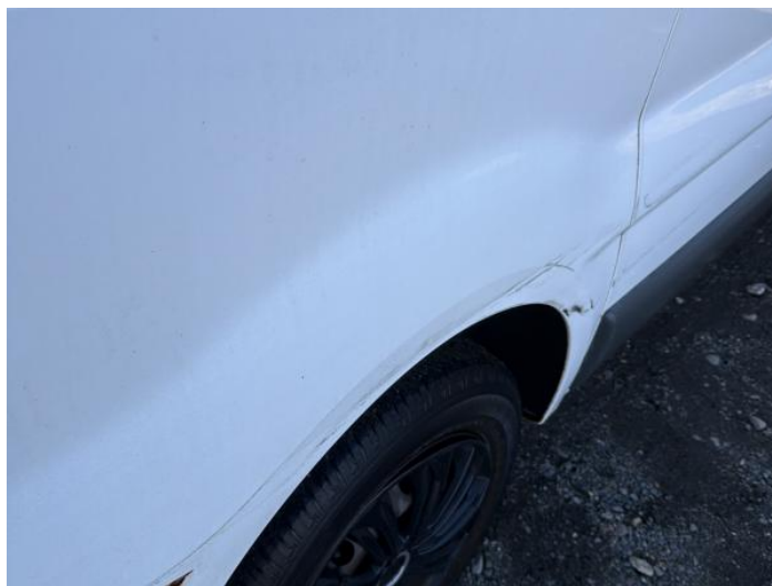
2: Qtr Panel or Dented With Paint Damage
