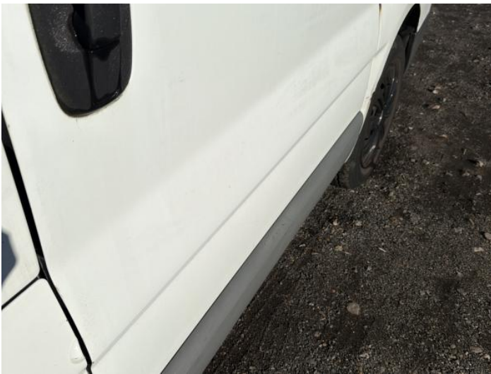
11: Door nsr Dented With Paint Damage
