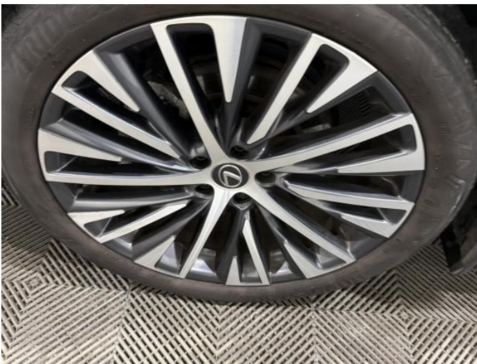
5: Wheel nsf Scratched Up To 50mm
