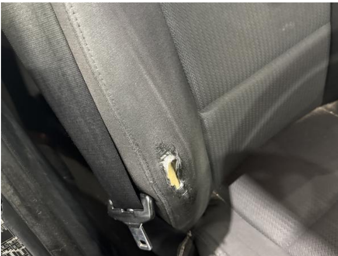
1: Seat Back Cover osf Holed Over 3mm
