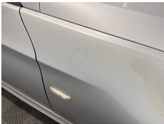
20: Wing osf Scratched Over 25mm Thru Paint
