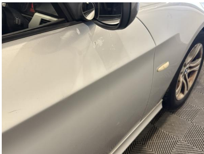
18: Door osf Dented With Paint Damage
