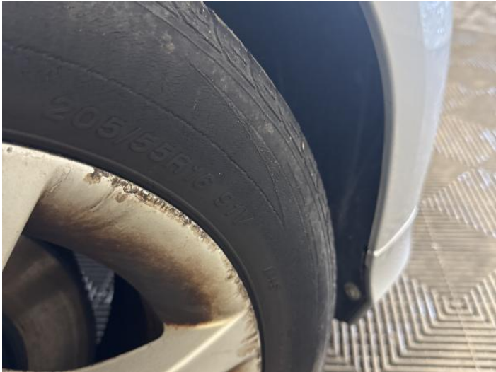
22: Tyre osf Damaged Replace
