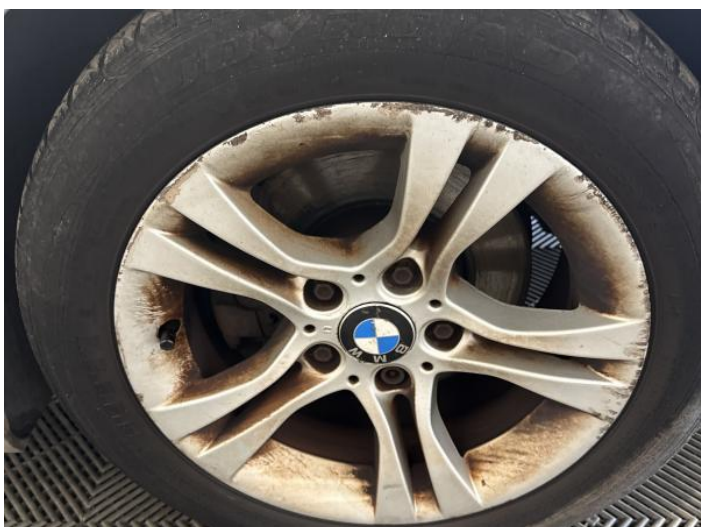
19: Wheel osf Scratched Over 50mm
