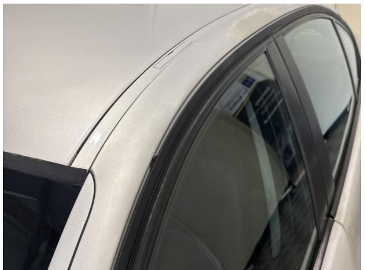
8: A Post ns Scratched Over 25mm Thru Paint
