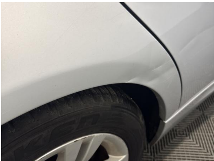
15: Qtr Panel osr Dented Over 30mm
