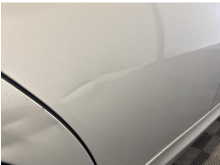
17: Door osr Dented Over 30mm
