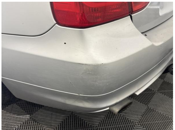
14: Bumper Rear Scratched Over 100mm Thru Paint
