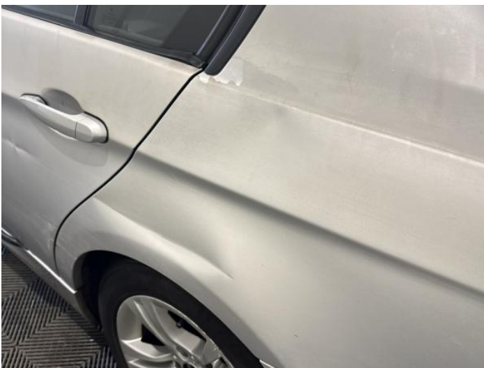
13: Qtr Panel nsr Dented With Paint Damage
