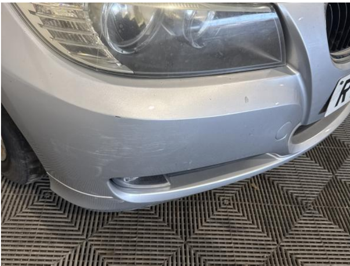
5: Bumper Front Scratched Over 100mm Thru Paint
