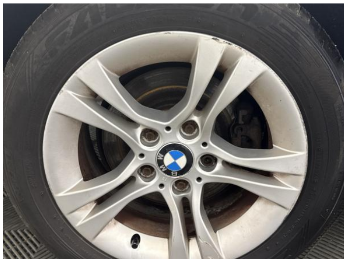
16: Wheel osr Scratched Over 50mm
