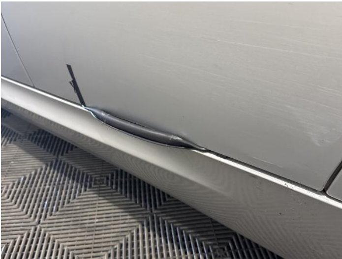
11: Aperture Seal nsr Broken Replace
