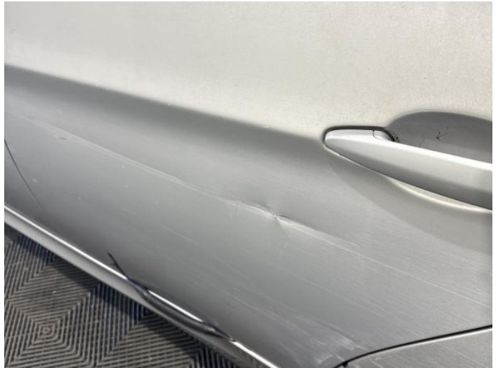
10: Door nsr Dented With Paint Damage
