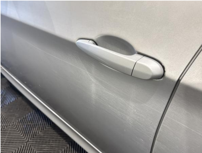
9: Door nsf Poor Previous Repair Poor Paint
