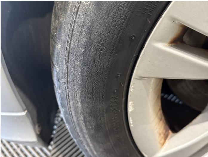
23: Tyre nsf Damaged Replace
