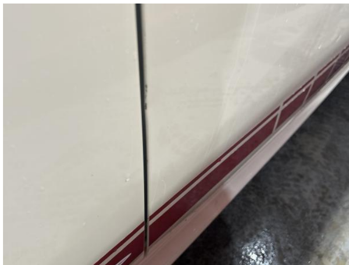
2: Door osf Chipped Edge Chip
