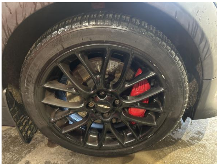
1: Wheel osf Scratched Over 50mm
