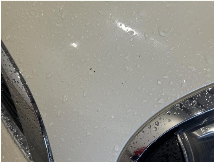
4: Bonnet Chipped Multiple Chips
