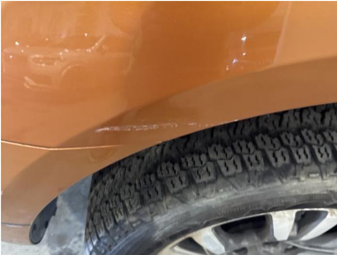
3: Wing nsf Scratched Over 25mm Thru Paint
