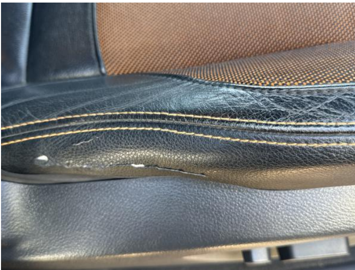
17: Seat Base Cover osf Torn Over 3mm
