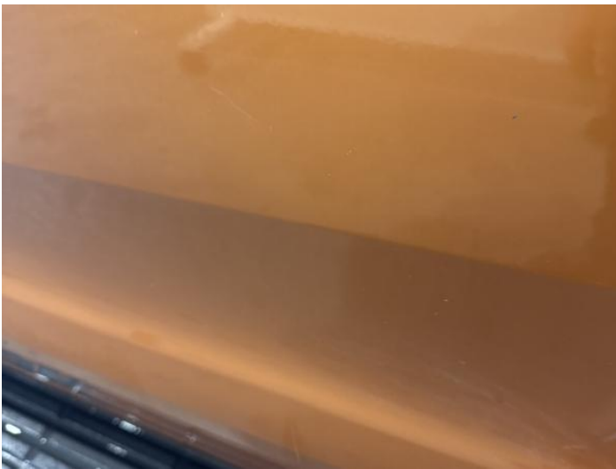
5: Door nsf Scratched Over 25mm Not Thru Paint
