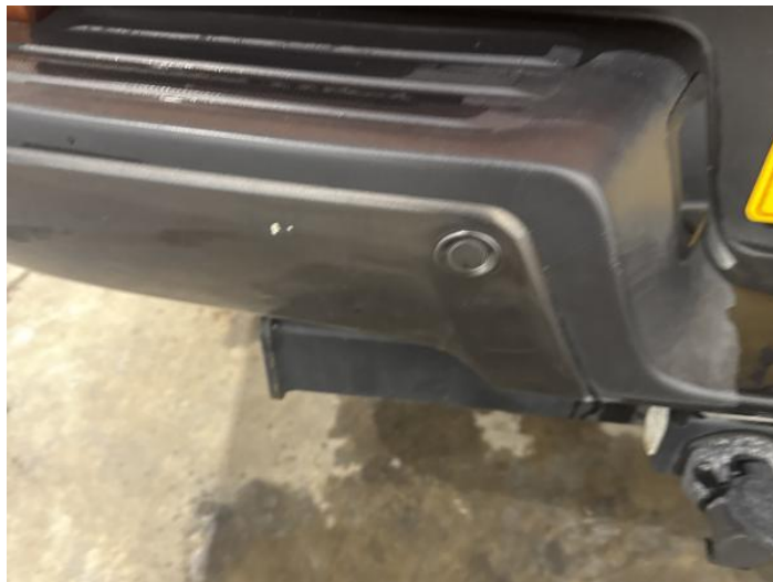
10: Bumper Rear Scratched Over 100mm Thru Paint
