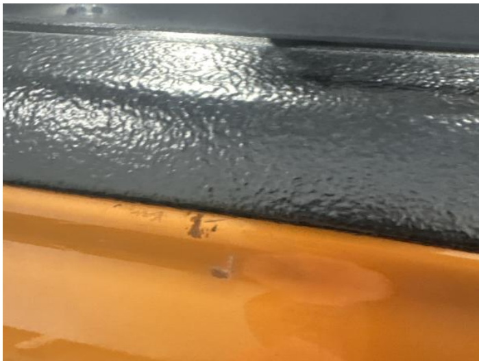
9: Boot Lid Dented With Paint Damage
