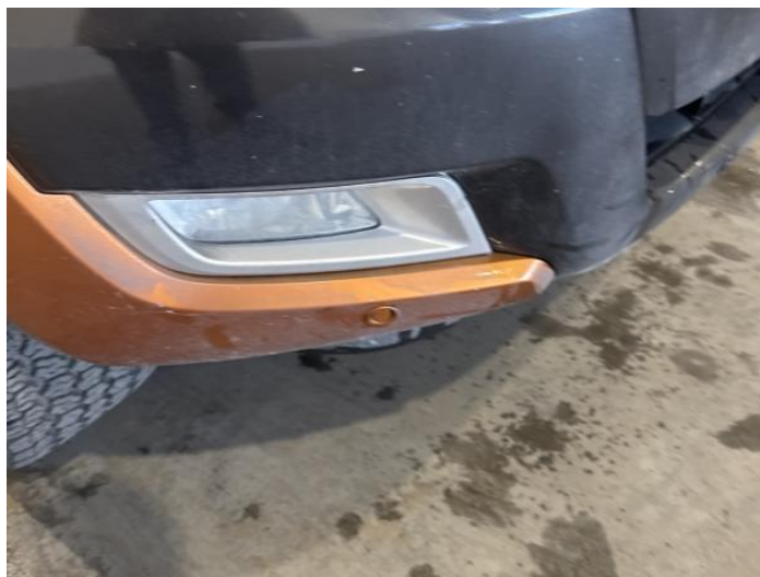
2: Bumper Front Scratched Over 100mm Thru Paint
