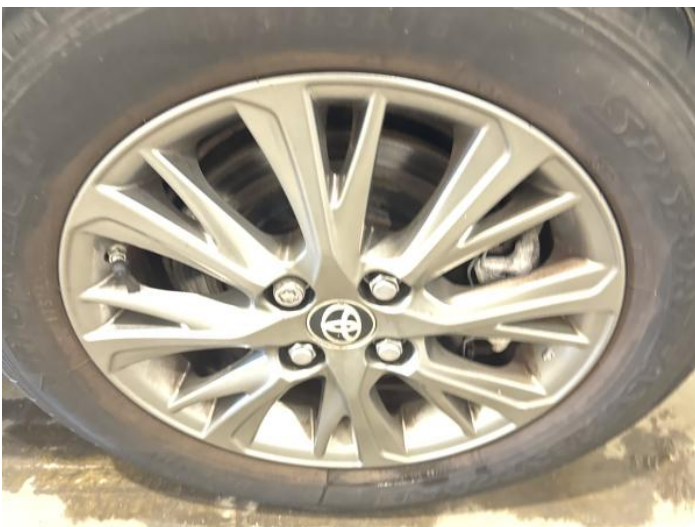
7: Wheel nsr Scratched Up To 50mm
