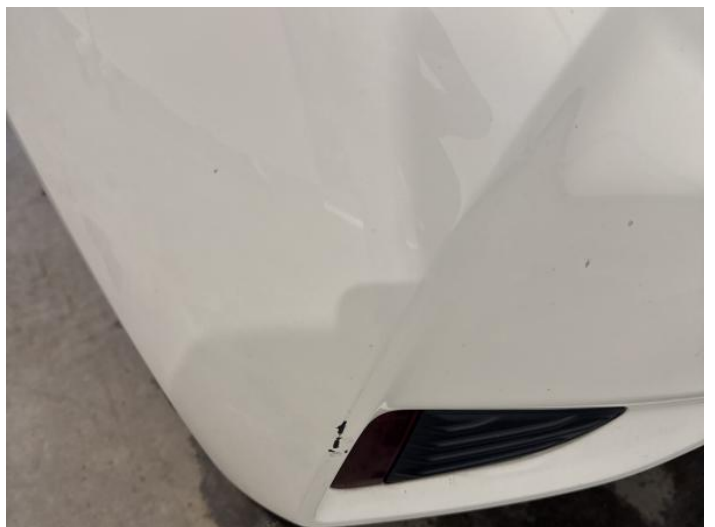
8: Bumper Rear Scratched 25 to 100mm Thru Paint
