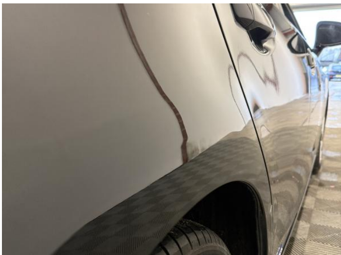
15: Qtr Panel osr Poor Previous Repair Poor Paint
