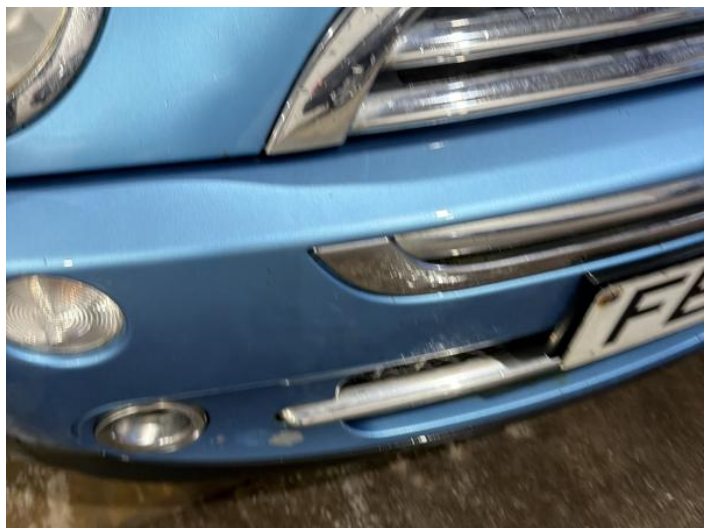
14: Bumper Front Poor Previous Repair Paint Flake
