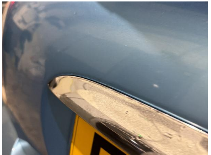
2: Boot Lid Dented Over 30mm
