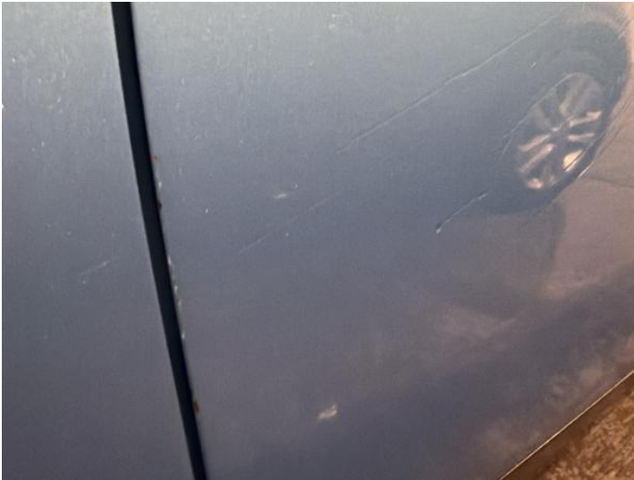
9: Door osf Chipped Edge Chip
