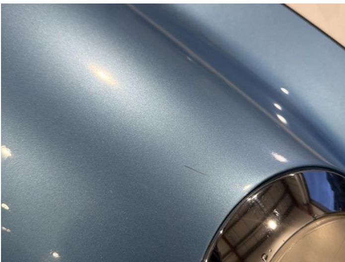
13: Bonnet Scratched Over 25mm Thru Paint
