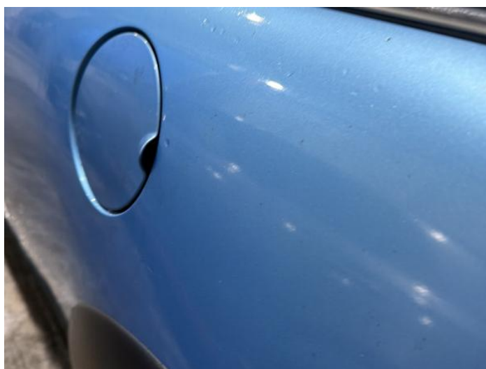
18: Qtr Panel nsr Dented Over 2 UpTo 10mm
