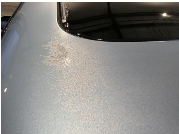
3: Roof Poor Previous Repair Poor Paint
