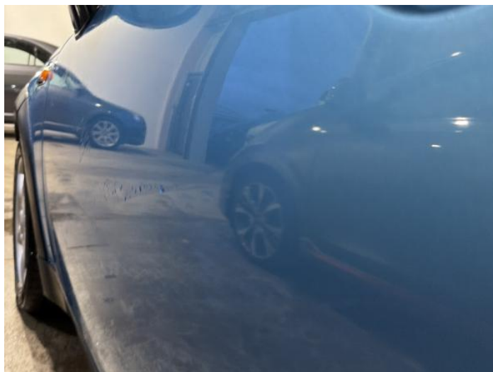
16: Door nsf Dented Over 2 UpTo 10mm
