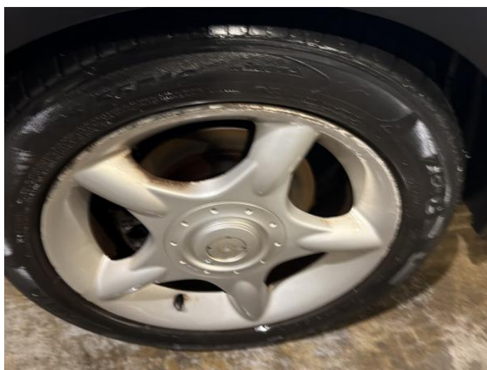
6: Wheel osr Scratched Over 50mm
