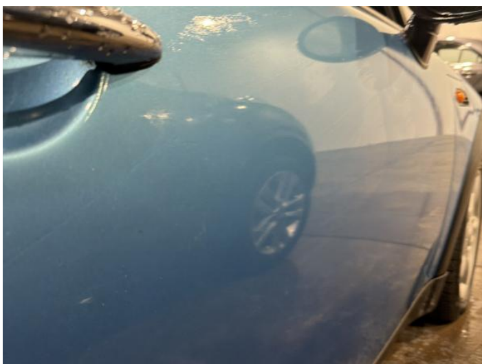
7: Door osf Dented Over 2 UpTo 10mm
