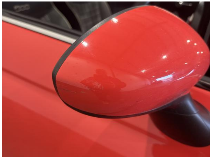
10: Door Mirror Assy osf Scratched (Painted) UpTo 25mm Thru Paint
