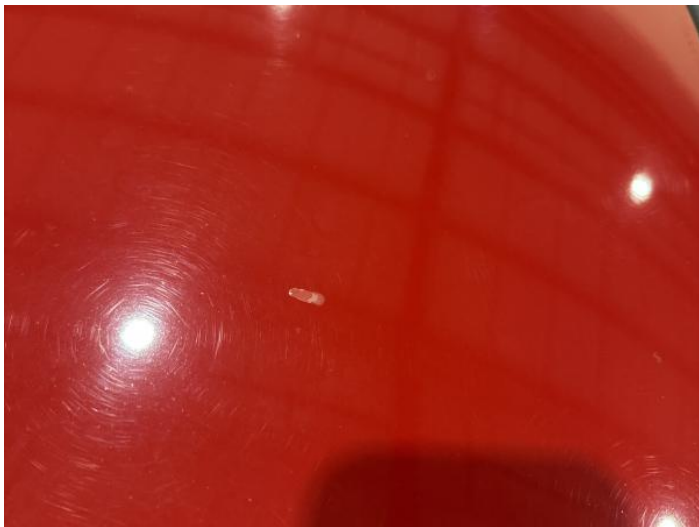
15: Roof Scratched UpTo 25mm Thru Paint
