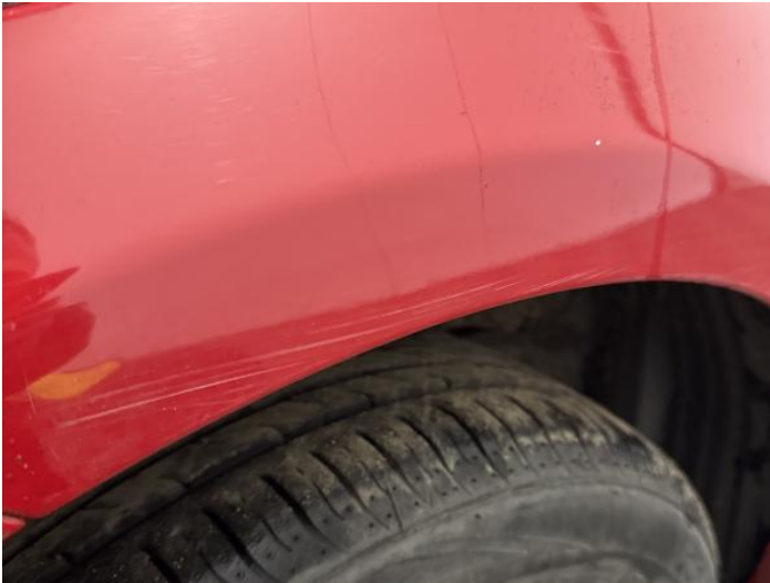
9: Qtr Panel osf Scratched Over 25mm Thru Paint
