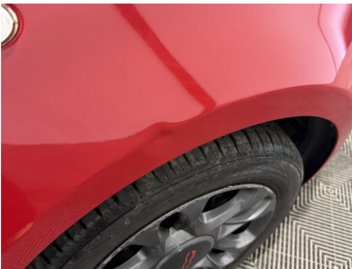
13: Wing osf Dented Over 30mm
