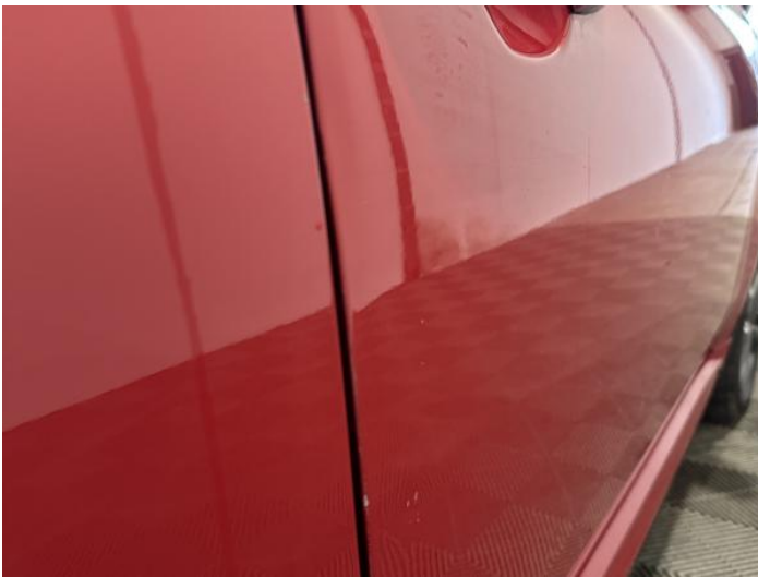
11: Door osf Dented With Paint Damage
