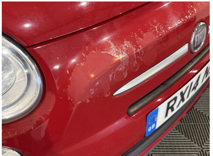
2: Bumper Front Poor Previous Repair Paint Flake
