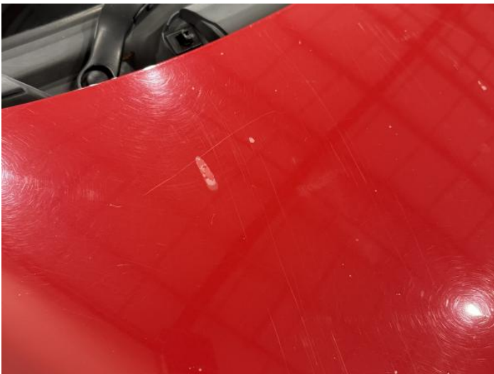
1: Bonnet Poor Previous Repair Paint Flake
