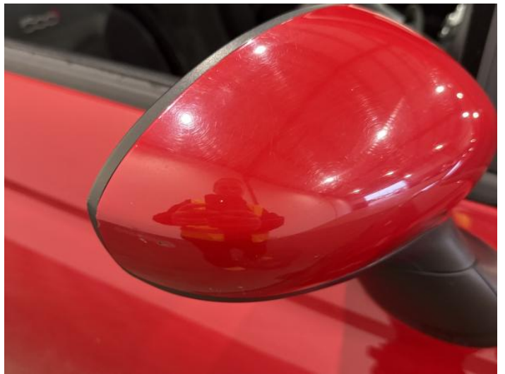
12: Door Mirror Assy osf Scratched (Painted) UpTo 25mm Thru Paint
