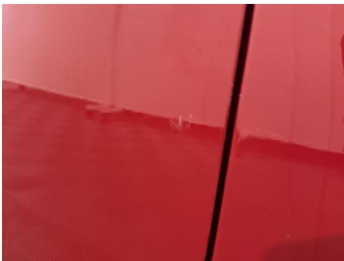
5: Door nsf Scratched UpTo 25mm Thru Paint
