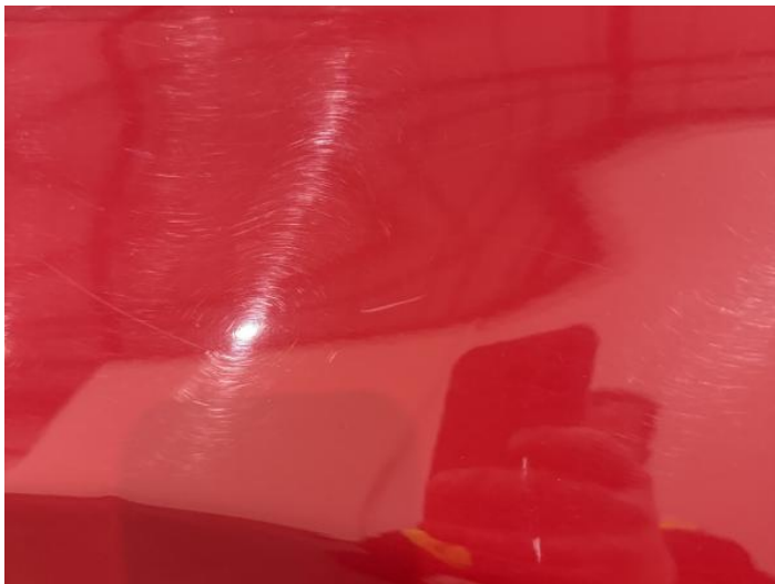
3: Wing nsf Scratched UpTo 25mm Thru Paint
