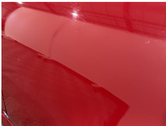
6: Qtr Panel nsr Dented Between 10mm + 30mm
