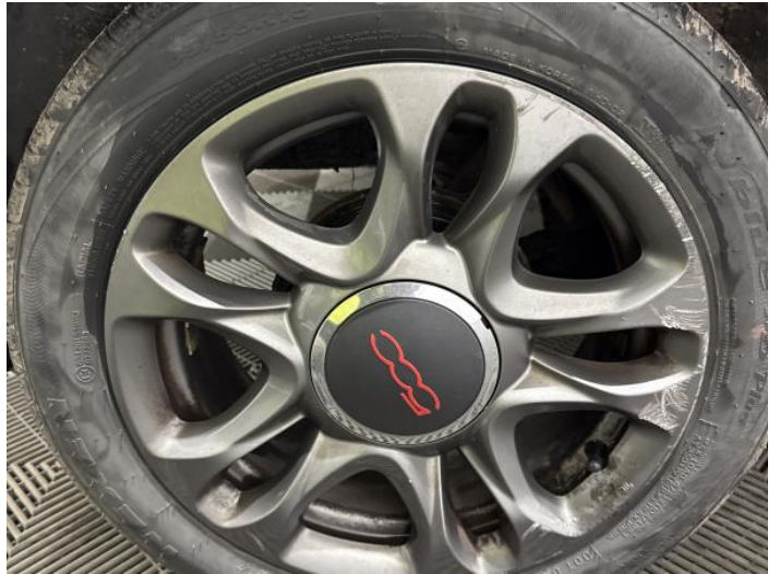
10: Wheel osf Scratched Over 50mm
