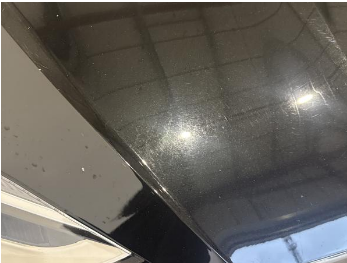
1: Bonnet Chipped Multiple Chips
