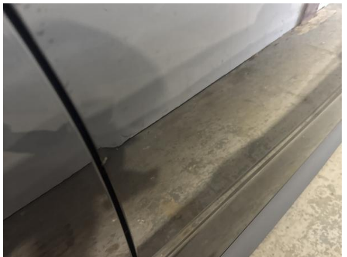
8: Door osf Dented Over 30mm
