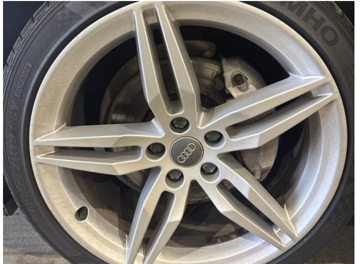
4: Wheel nsf Scratched Over 50mm
