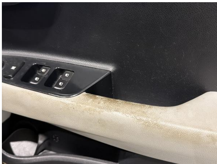
2: Door Pad osf Scuffed Over 25mm
