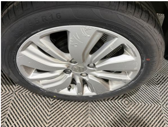
11: Wheel nsr Scratched Over 50mm
