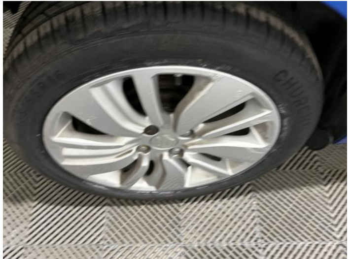
16: Wheel osr Scratched Over 50mm
