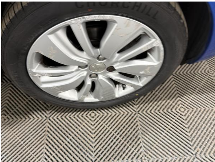
23: Wheel osf Scratched Over 50mm
