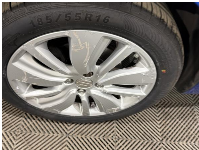
4: Wheel nsf Scratched Over 50mm
