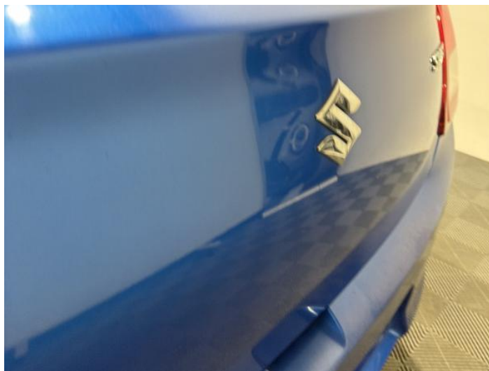
14: Boot Lid Dented Over 2 UpTo 10mm
