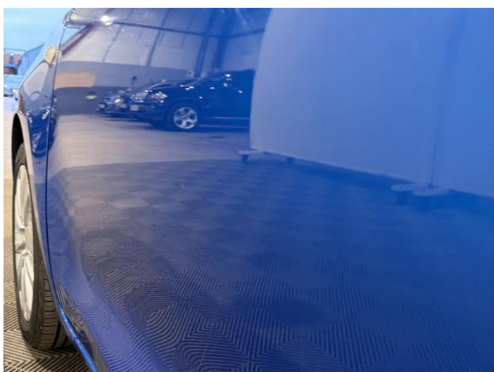
7: Door nsf Dented Over 2 UpTo 10mm
