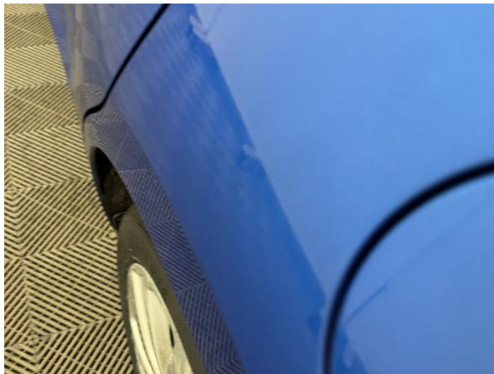
12: Qtr Panel nsr Dented Over 2 UpTo 10mm
