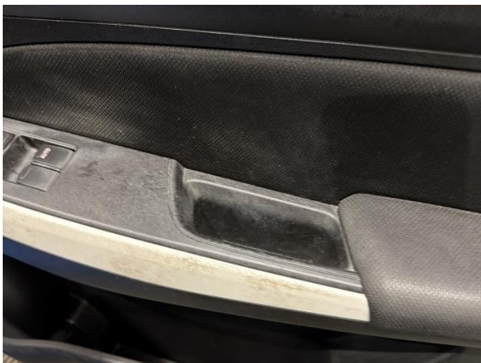
1: Door Pad osf Scuffed UpTo 25mm
