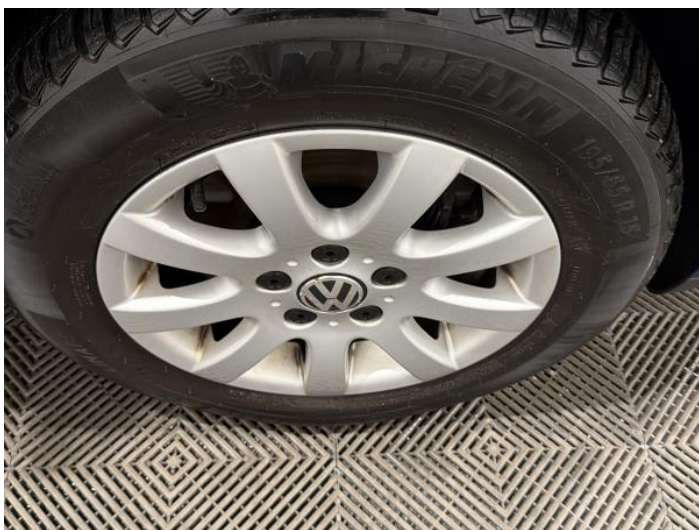
23: Wheel of Scratched Up To 50mm
