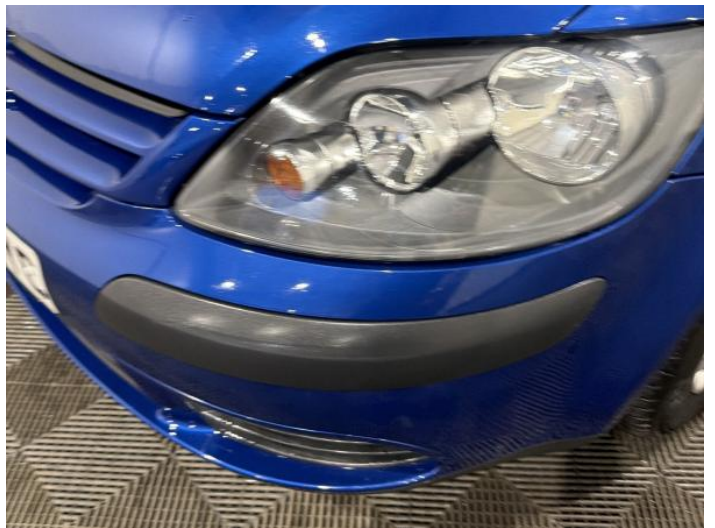
2: Bumper Front Chipped Multiple Chips
