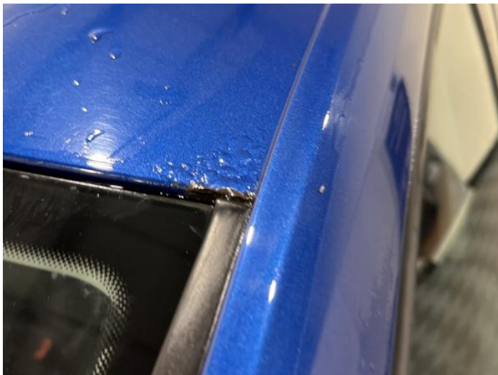
21: Roof Rusted Over 5mm
