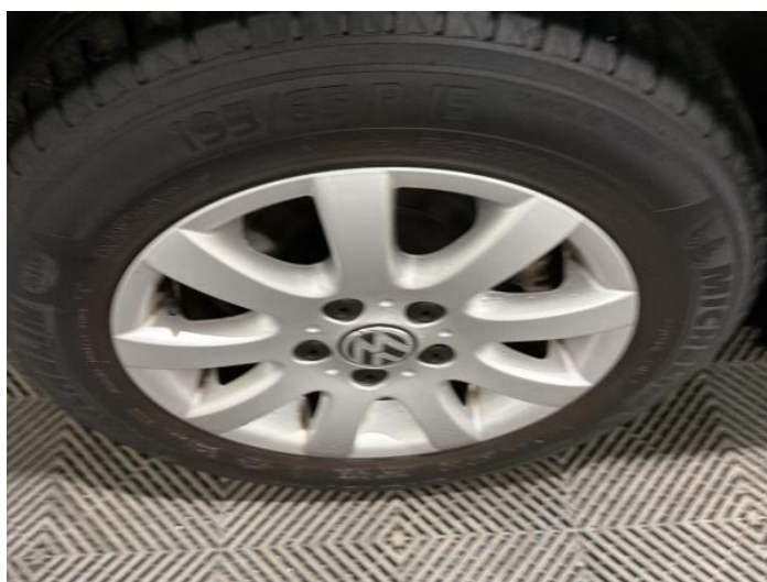
18: Wheel osr Scratched Up To 50mm
