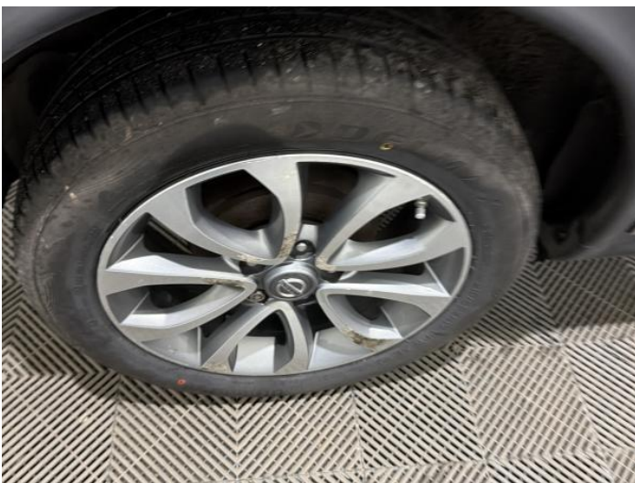
13: Wheel osr Scratched Over 50mm
