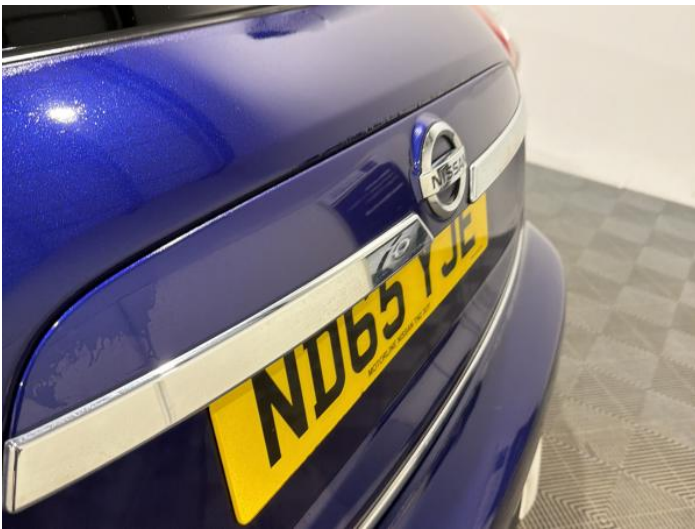
11: Boot Lid Dented Over 2 UpTo 10mm
