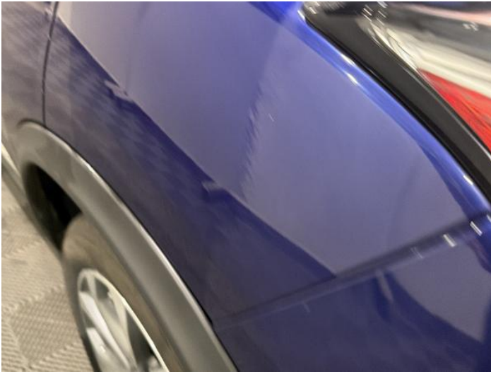
9: Qtr Panel nsr Dented Over 2 UpTo 10mm
