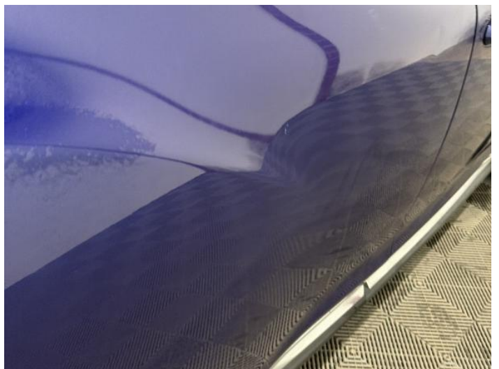
14: Door osr Dented With Paint Damage
