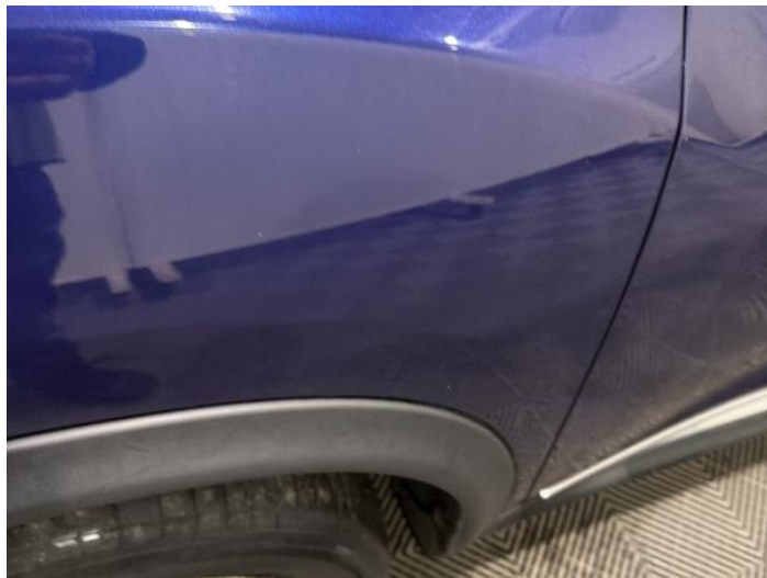
4: Wing nsf Dented Over 2 UpTo 10mm
