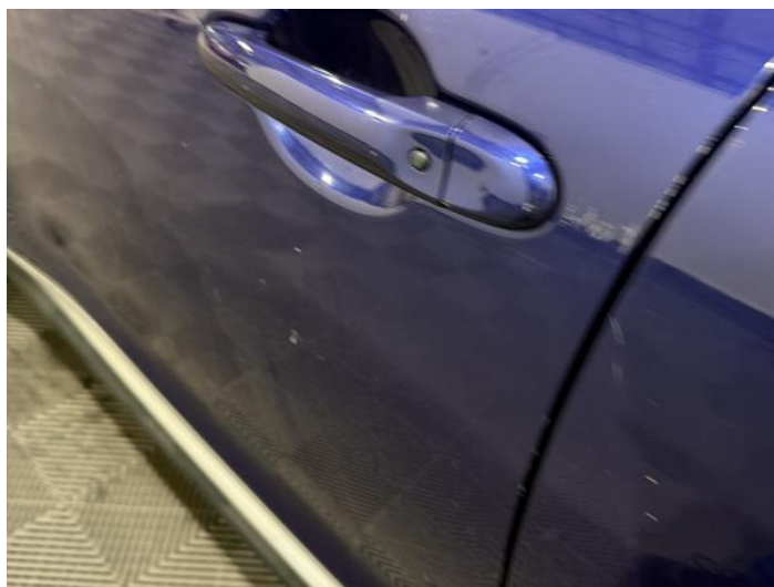
6: Door nsf Dented With Paint Damage
