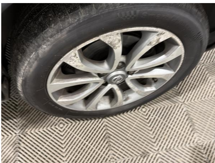
17: Wheel osf Scratched Over 50mm
