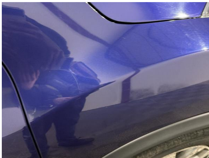
16: Wing osf Dented With Paint Damage
