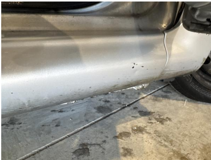
11: Sill os Dented With Paint Damage
