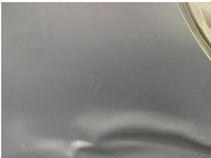
3: Wing osf Dented Over 30% Of Panel
