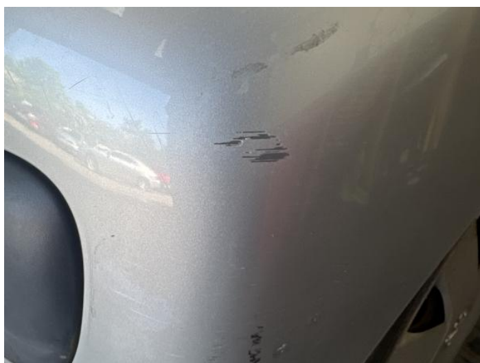
6: Bumper Rear Scratched Over 100mm Thru Paint
