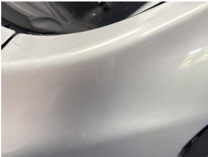
9: Wing nsf Poor Previous Repair Poor Paint
