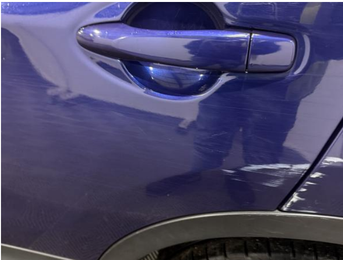
7: Door nsr Dented With Paint Damage
