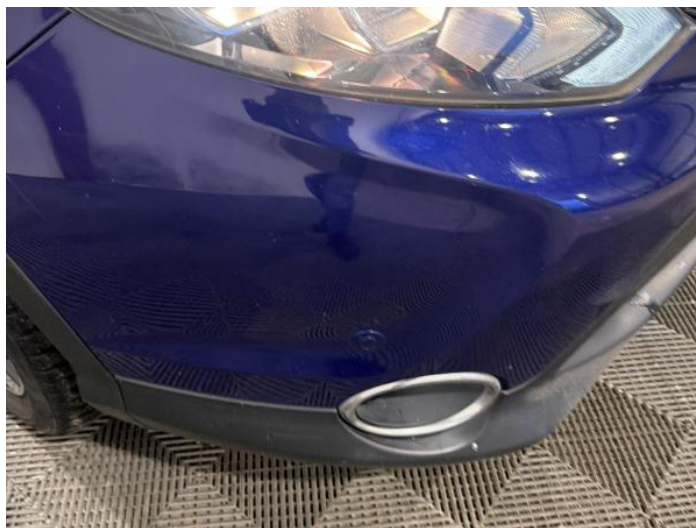
2: Bumper Front Poor Previous Repair Poor Paint
