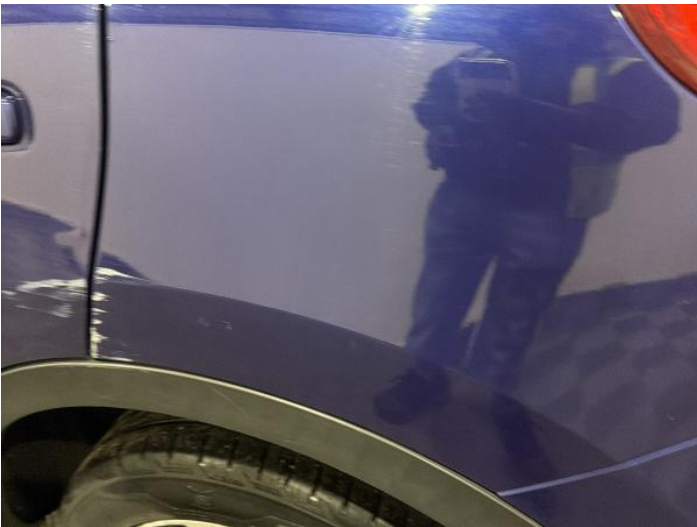
8: Qtr Panel nsr Dented With Paint Damage
