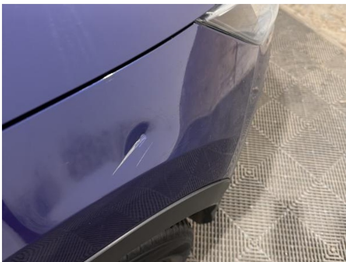
17: Wing osf Dented With Paint Damage
