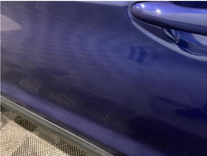
6: Door nsf Dented With Paint Damage
