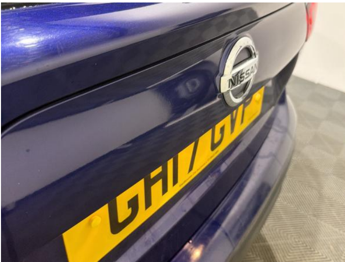
11: Boot Lid Dented Over 2 UpTo 10mm
