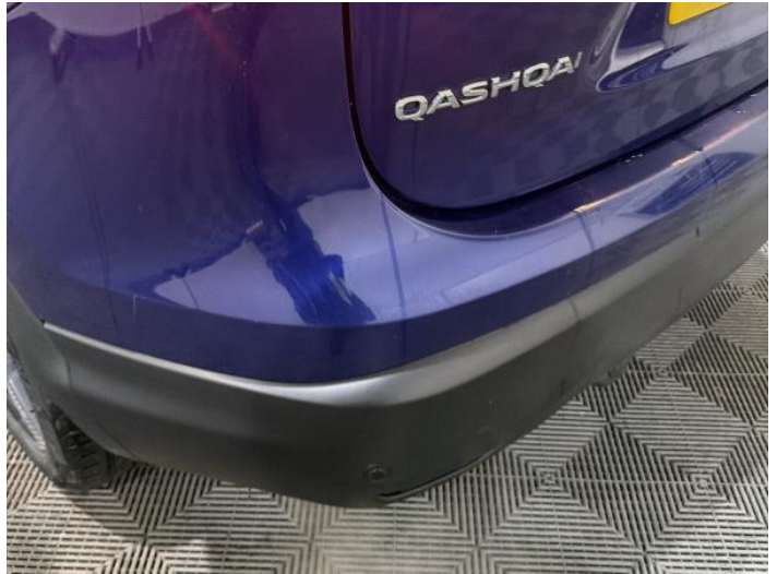
10: Bumper Rear Scratched Over 100mm Thru Paint
