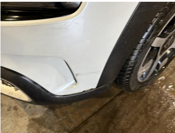
13: Bumper Front Moulding Broken Replace
