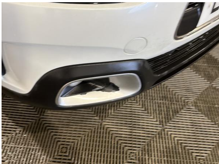
21: Bumper Front Moulding Scratched (Painted) Over 25mm Thru Paint
