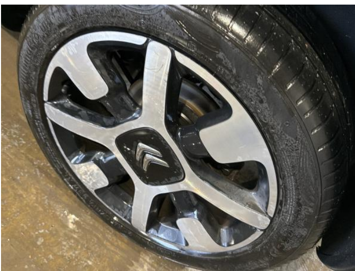
19: Wheel nsr Scratched Up To 50mm
