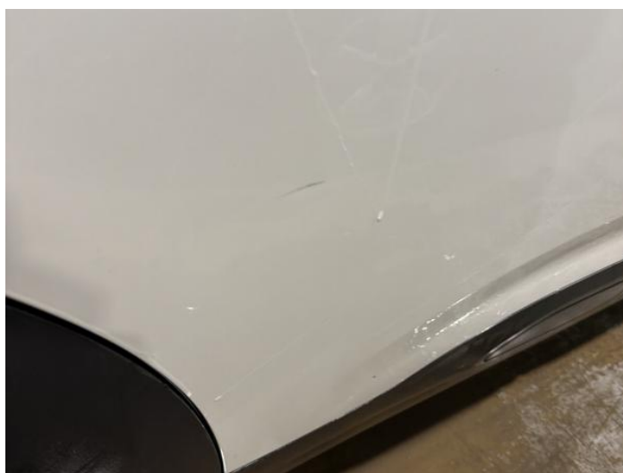
6: Door osr Dented Between 10mm + 30mm
