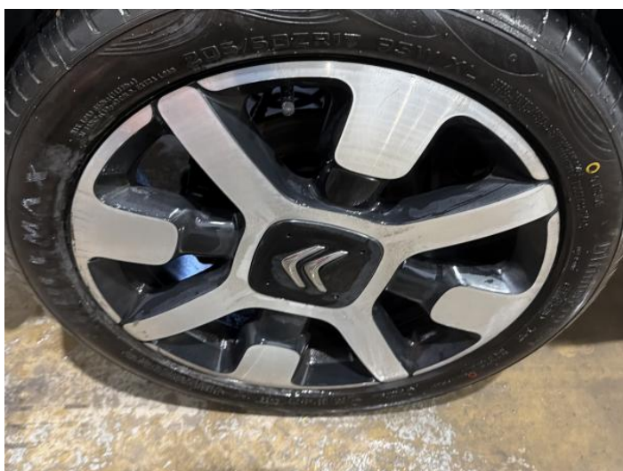
5: Wheel osr Scratched Over 50mm
