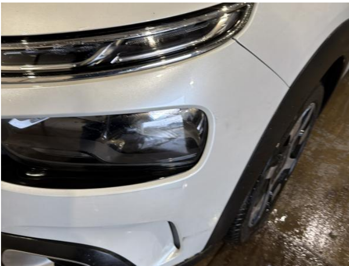
11: Bumper Front Scratched 25 to 100mm Thru Paint
