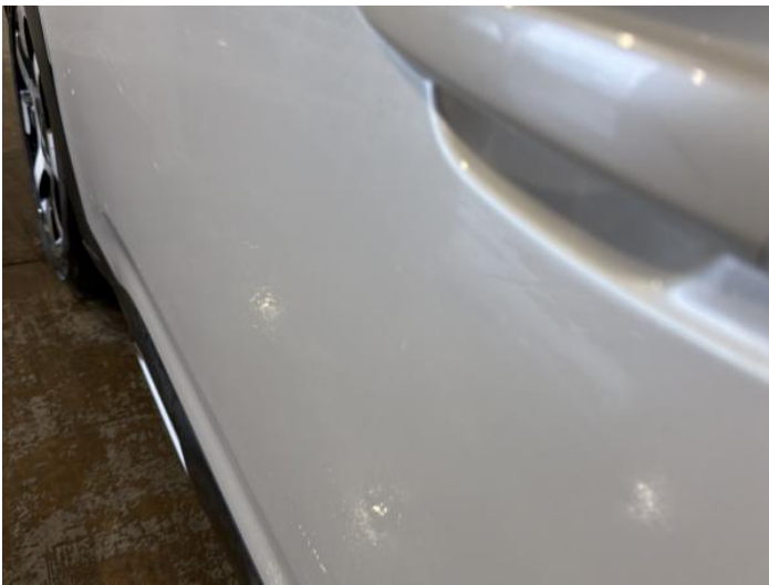
17: Door nsf Dented Over 2 UpTo 10mm
