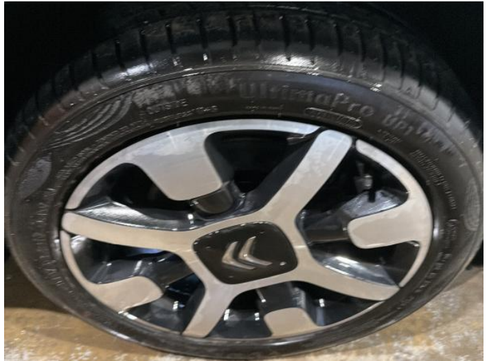
10: Wheel osf Scratched Up To 50mm
