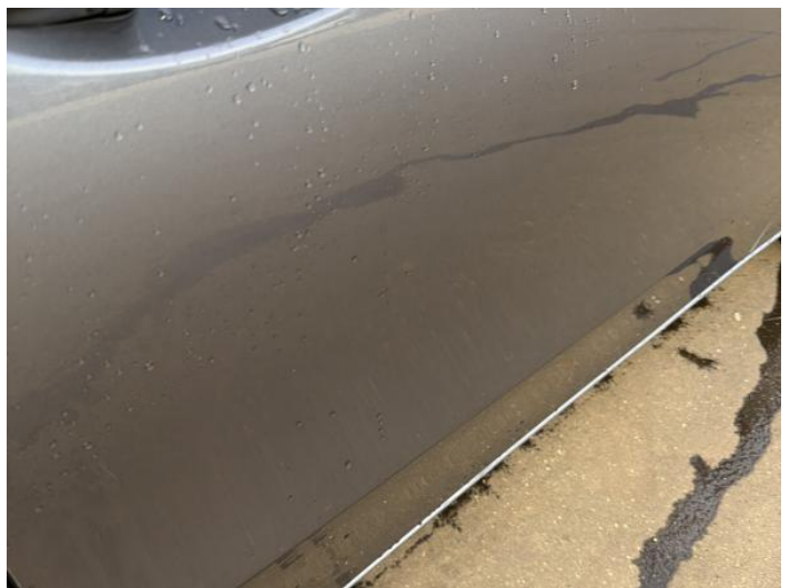
8: Door osf Dented Over 2 UpTo 10mm
