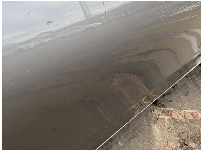
16: Door nsf Scratched Over 25mm Thru Paint
