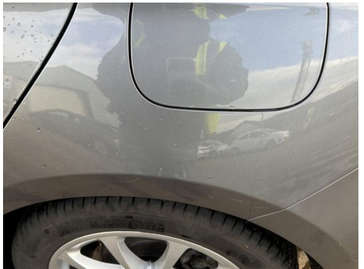
18: Qtr Panel nsr Poor Previous Repair Poor Paint
