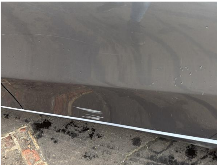
17: Door nsr Dented With Paint Damage
