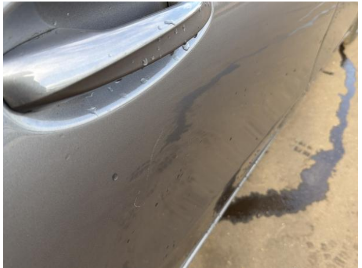
6: Door osr Scratched Over 25mm Thru Paint
