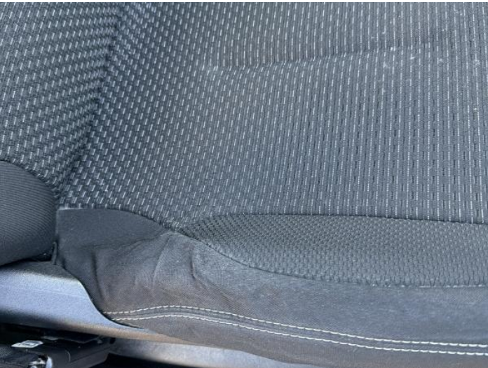
1: Seat Base Cover osf Scuffed UpTo 25mm
