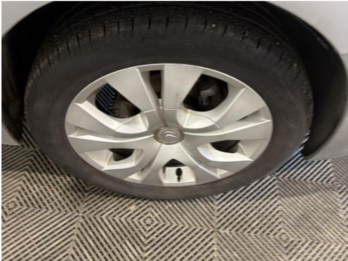
22: Wheel osf Scratched Over 50mm
