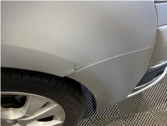
21: Wing osf Cracked Replace
