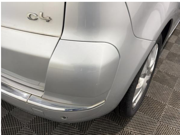
15: Bumper Rear Scratched Over 100mm Thru Paint
