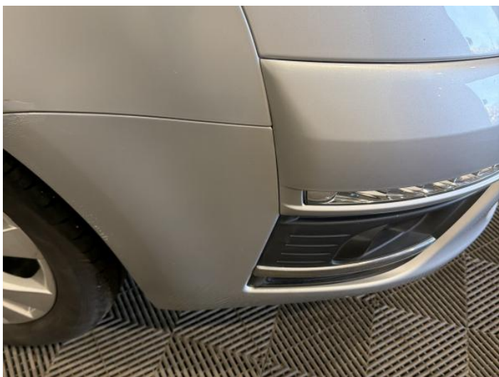
5: Bumper Front Poor Previous Repair Poor Paint
