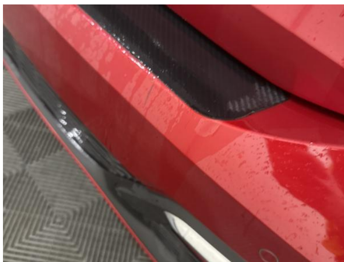
8: Bumper Rear Scratched Up To 25mm Thru Paint
