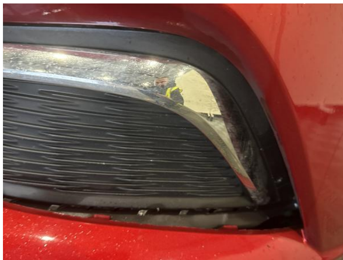
2: Bumper Front Grill Broken Replace
