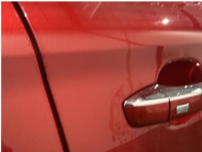
11: Door osf Scratched UpTo 25mm Thru Paint
