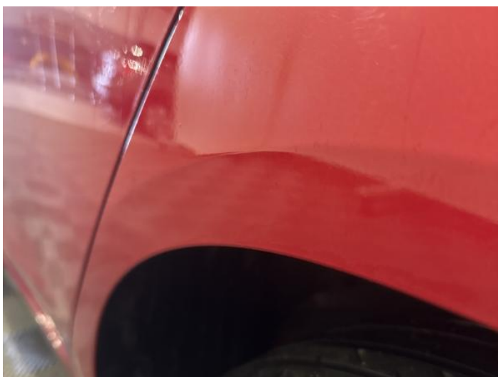
7: Qtr Panel nsr Dented Between 10mm + 30mm
