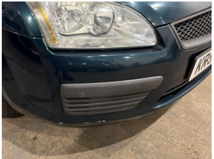
2: Bumper Front Scratched Over 100mm Thru Paint
