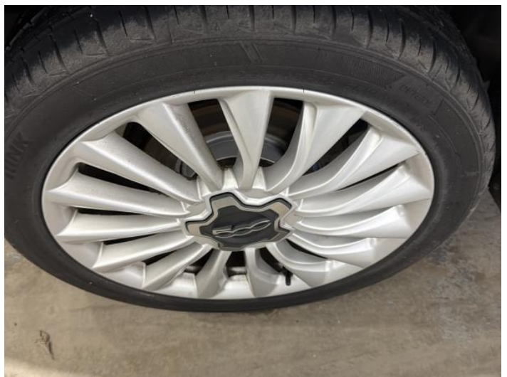
14: Wheel osr Scratched Up To 50mm
