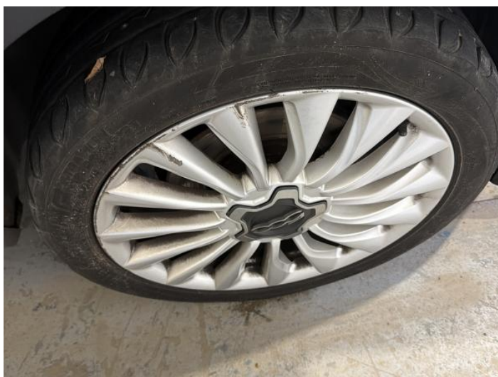
19: Wheel osf Scratched Over 50mm
