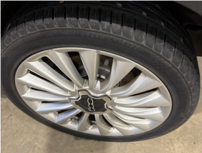
9: Wheel nsr Scratched Up To 50mm
