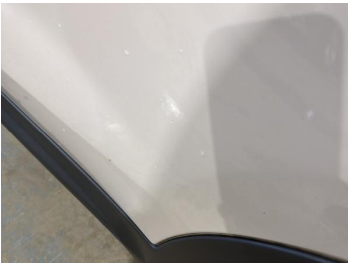
7: Door nsr Dented 2 Or Less UpTo 10mm
