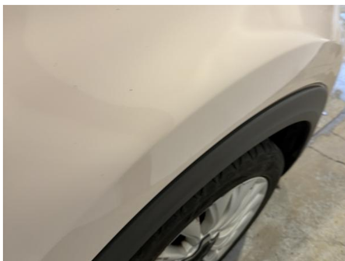
18: Wing osf Dented Over 2 UpTo 10mm
