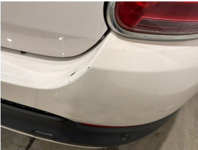
11: Bumper Rear Cracked UpTo 25mm
