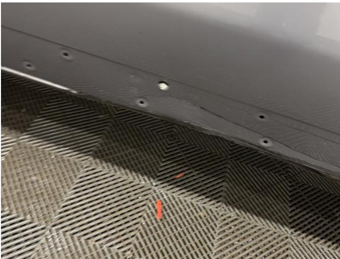
17: Sill ns Dented With Paint Damage
