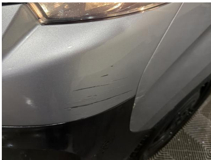
12: Bumper Front Scratched 25 to 100mm Thru Paint
