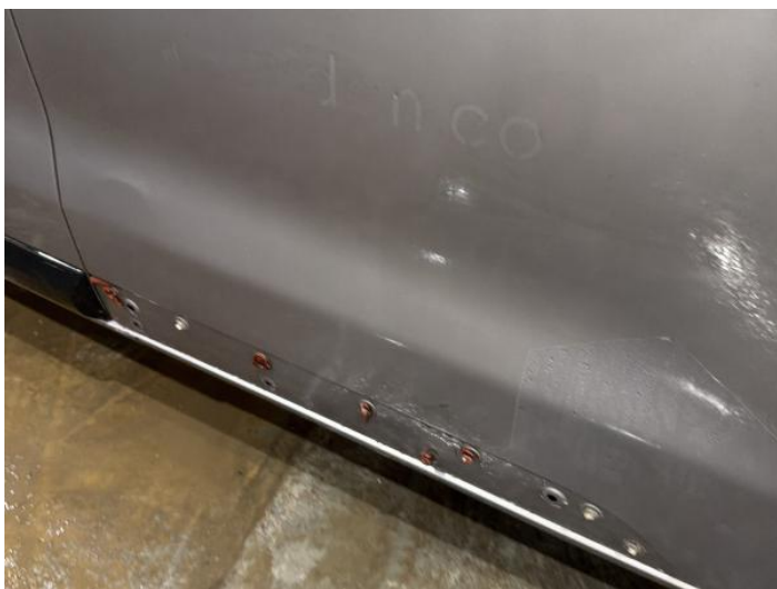
5: Door Moulding osf Missing Replace
