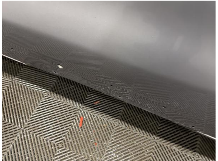
16: Door nsr Dented With Paint Damage
