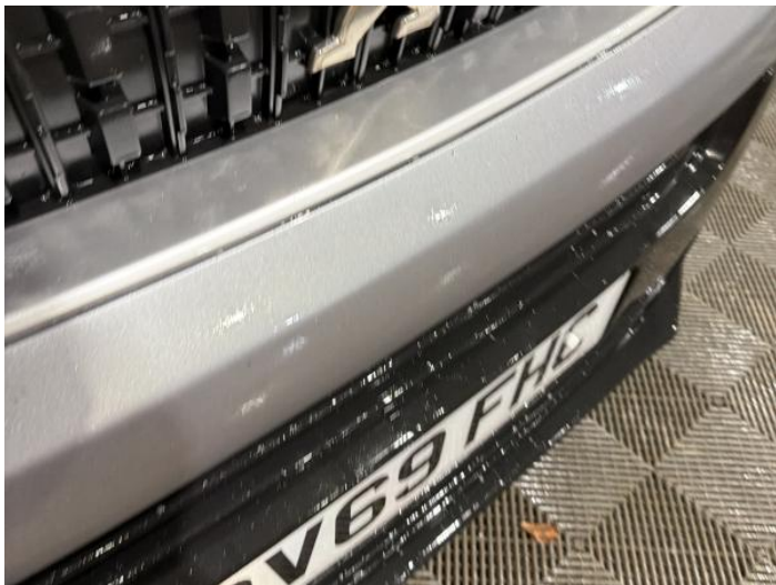
9: Bumper Front Chipped Multiple Chips
