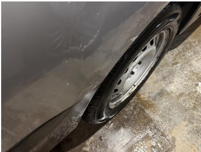
3: Qtr Panel osr Dented Over 30mm
