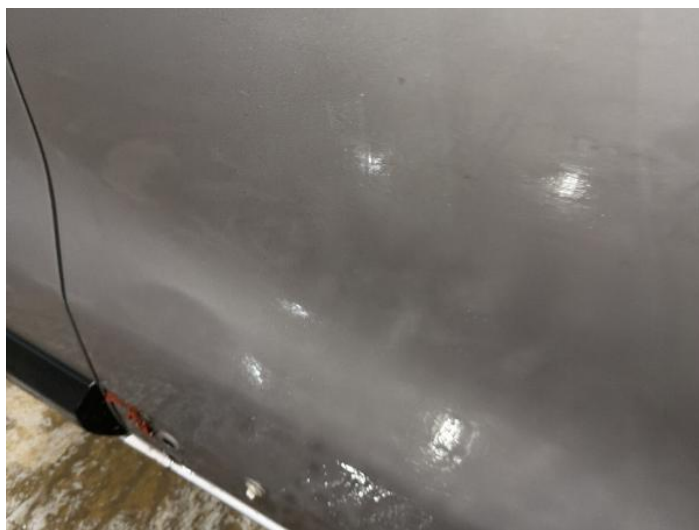
6: Door osf Dented Over 30mm
