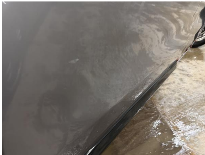
4: Door osr Dented Over 30mm
