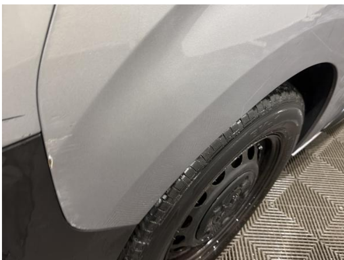
13: Wing nsf Dented With Paint Damage
