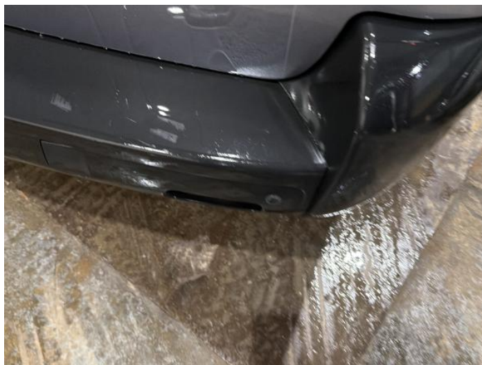
2: Bumper Rear Moulding Scuffed (Unpainted) UpTo 100mm
