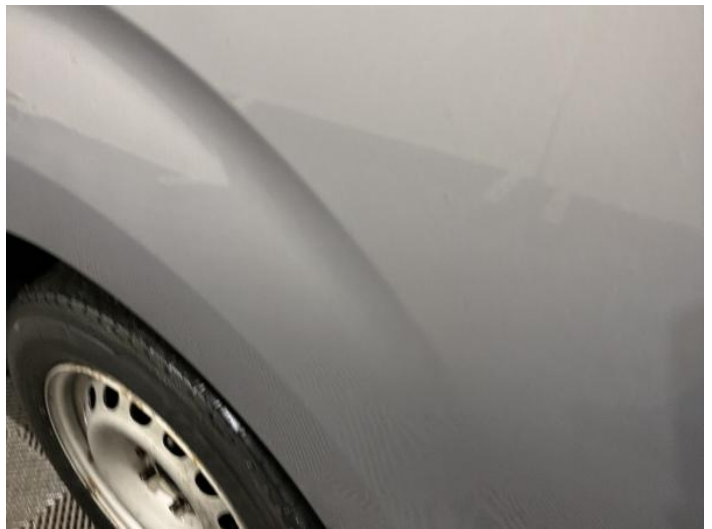
18: Qtr Panel nsr Dented Over 2 UpTo 10mm
