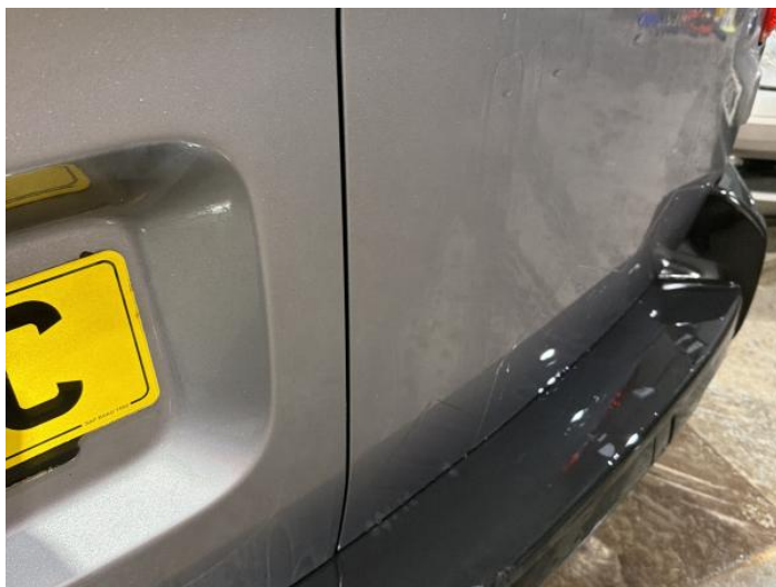
1: Boot Lid Dented Over 30mm
