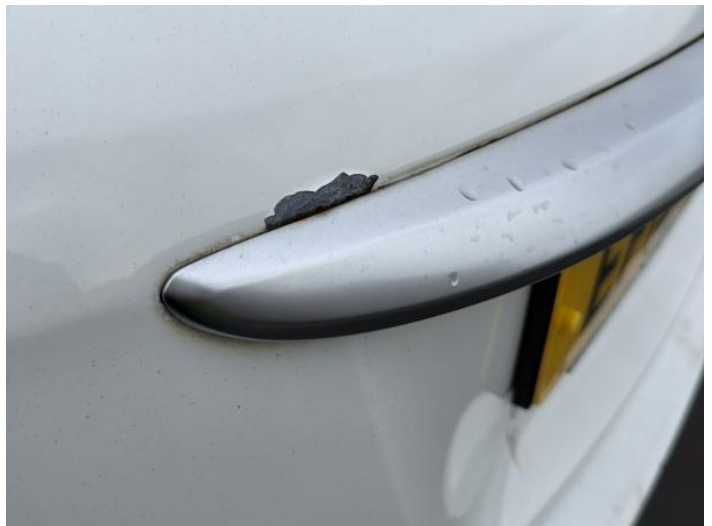
2: Boot Lid Poor Previous Repair Paint Flake
