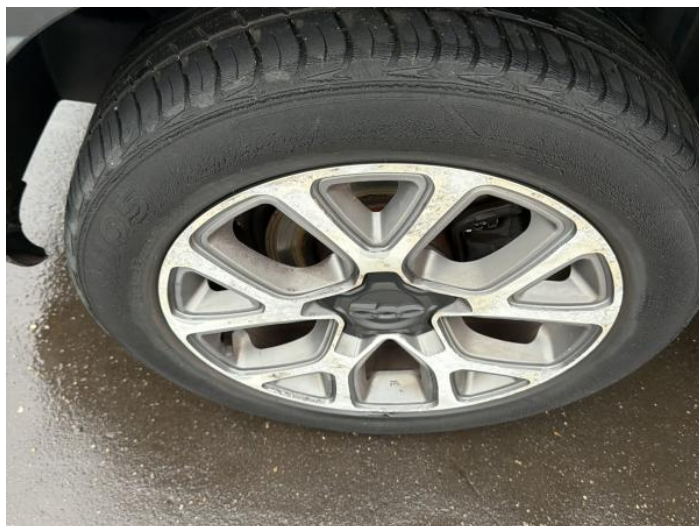
4: Wheel osr Scratched Over 50mm
