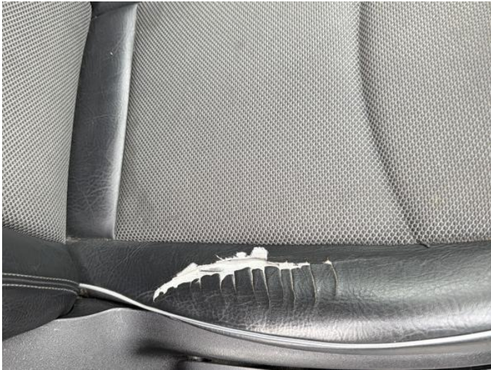
22: Seat Base Cover osf Torn Over 3mm
