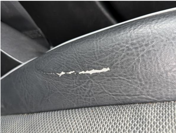
23: Seat Base Cover nsf Torn Over 3mm
