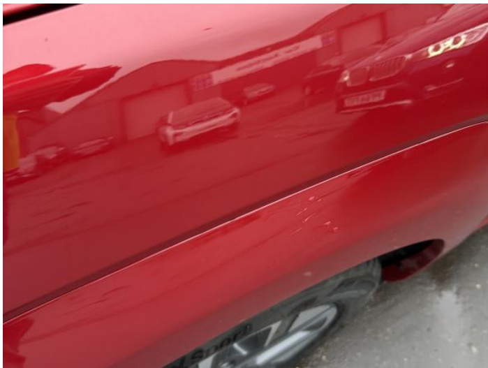
15: Wing nsf Dented Over 2 Up To 10mm
