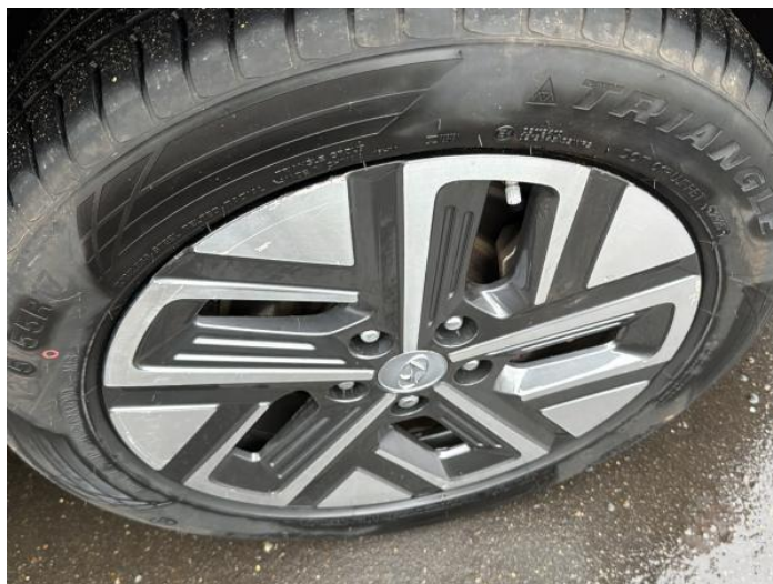
10: Wheel osf Scratched Over 50mm
