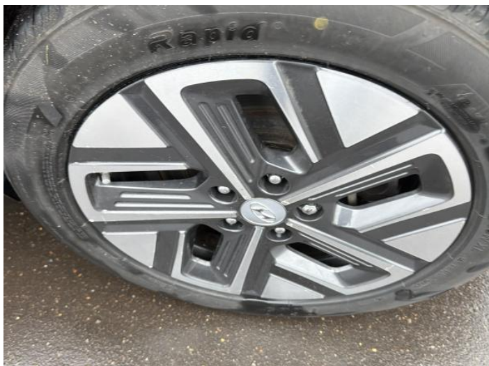
21: Wheel nsr Scratched Up To 50mm
