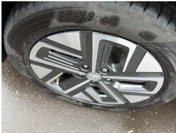
16: Wheel nsf Scratched Up To 50mm
