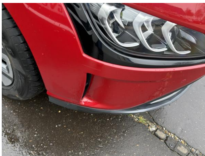
12: Bumper Front Scratched UpTo 25mm Thru Paint
