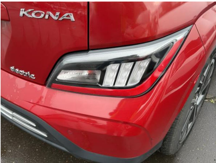
1: Bumper Rear Scratched 25 to 100mm Thru Paint
