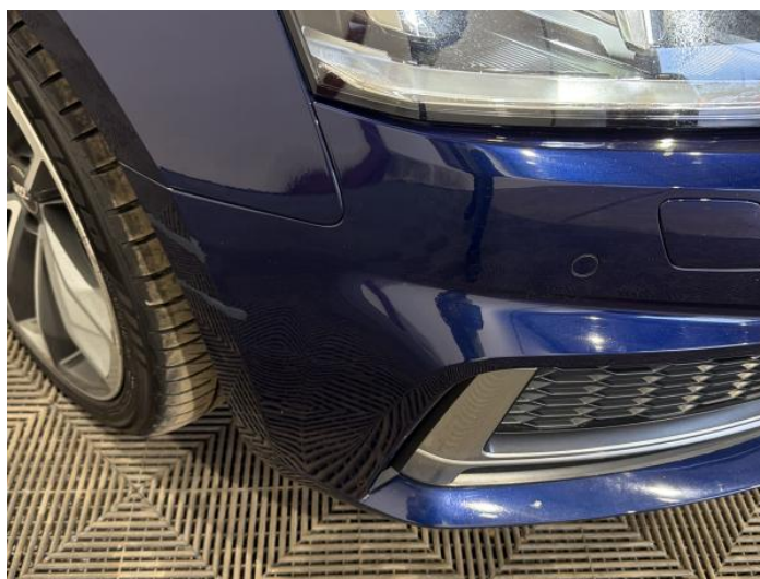
2: Bumper Front Scratched 25 to 100mm Thru Paint
