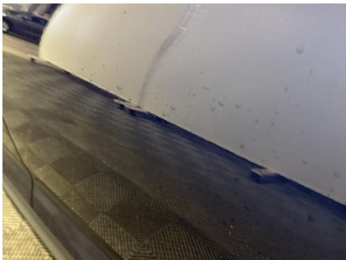
9: Door nsr Dented 2 Or Less UpTo 10mm
