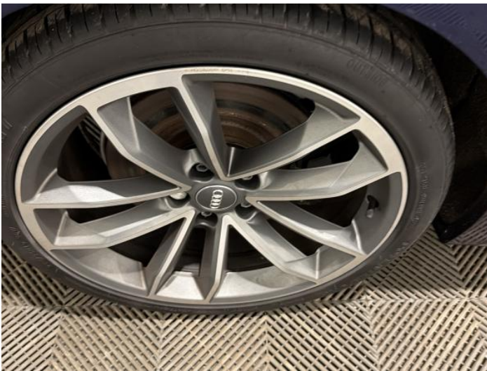
17: Wheel osr Scratched Up To 50mm
