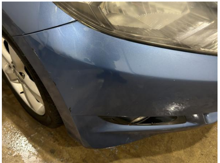
2: Bumper Front Scratched Over 100mm Thru Paint
