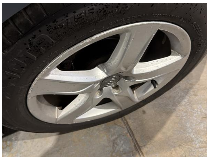
26: Wheel osf Scratched Over 50mm
