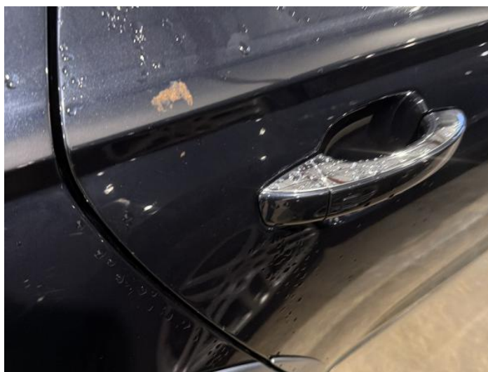
20: Door osr Rusted Over 5mm
