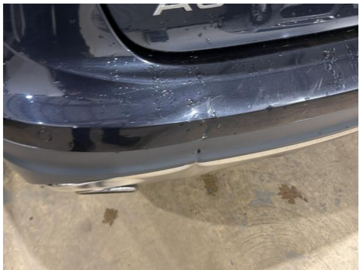
14: Bumper Rear Moulding Broken Replace
