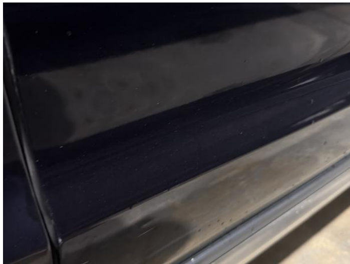
22: Door osf Scratched UpTo 25mm Thru Paint
