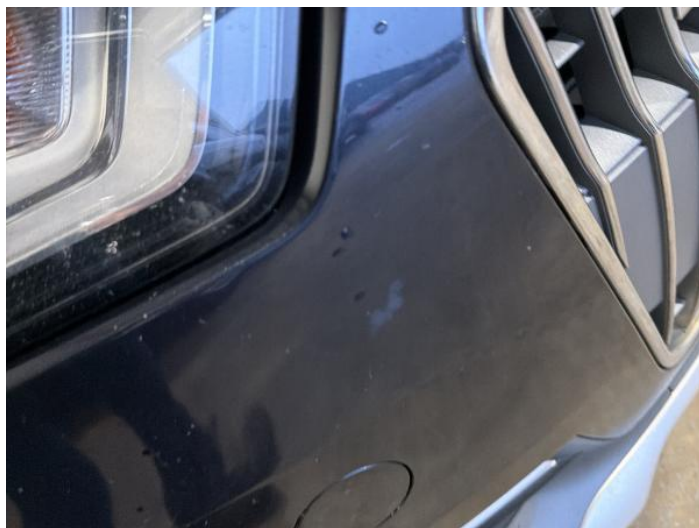
2: Bumper Front Poor Previous Repair Poor Paint
