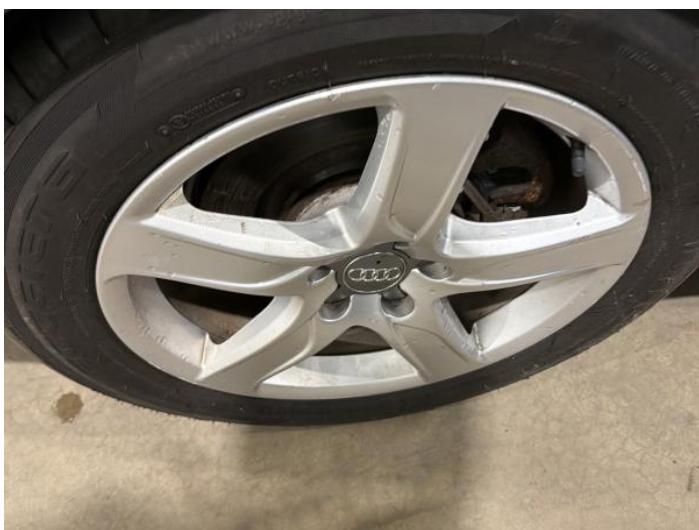
19: Wheel osr Scratched Over 50mm
