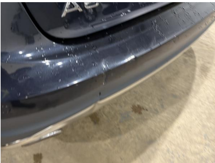
13: Bumper Rear Dented With Paint Damage
