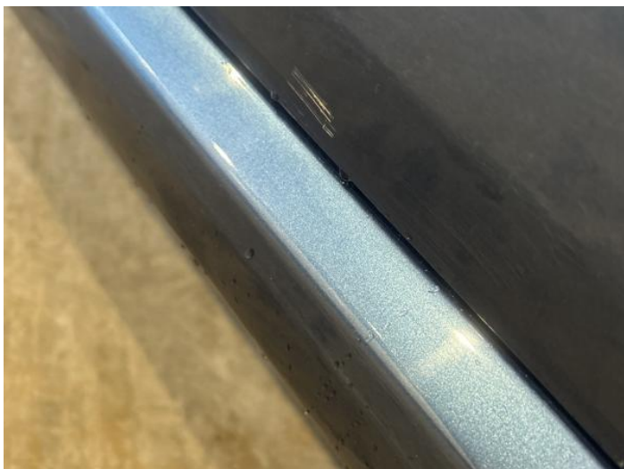
3: Door nsr Scratched UpTo 25mm Thru Paint
