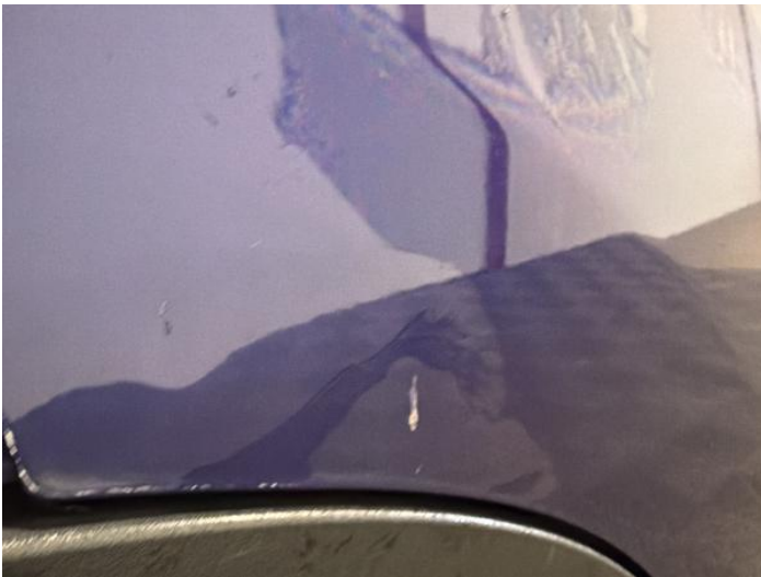
19: Door osr Dented Over 2 UpTo 10mm
