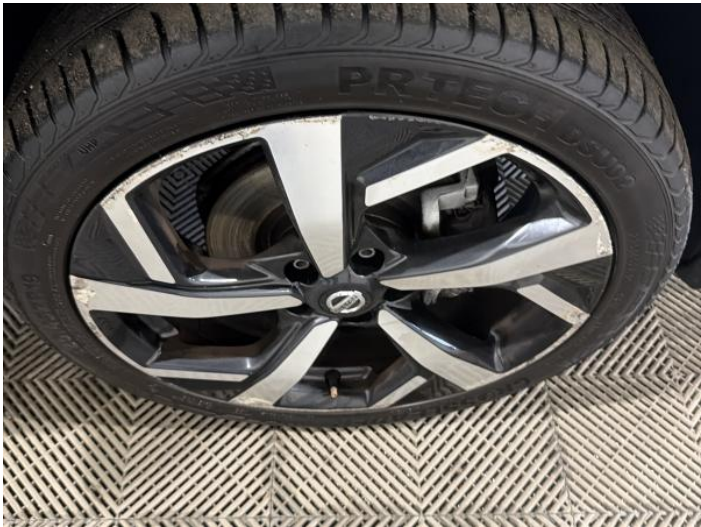
24: Wheel osf Scratched Over 50mm
