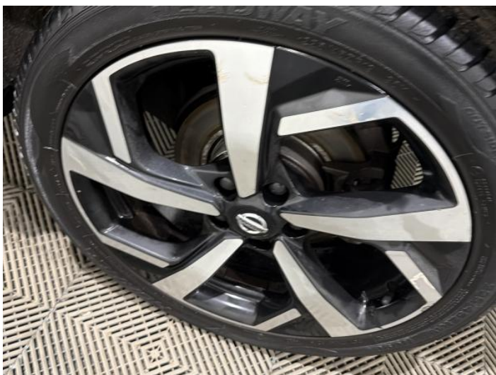
11: Wheel nsr Scratched Over 50mm
