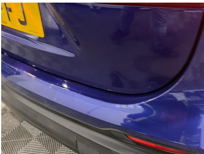
13: Bumper Rear Chipped Multiple Chips
