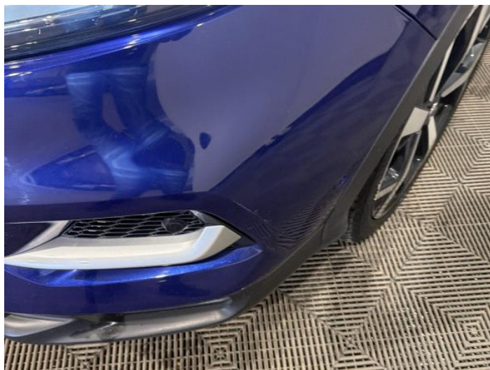
2: Bumper Front Scratched 25 to 100mm Thru Paint
