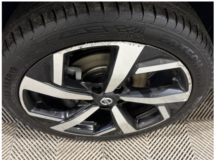
6: Wheel nsf Scratched Over 50mm
