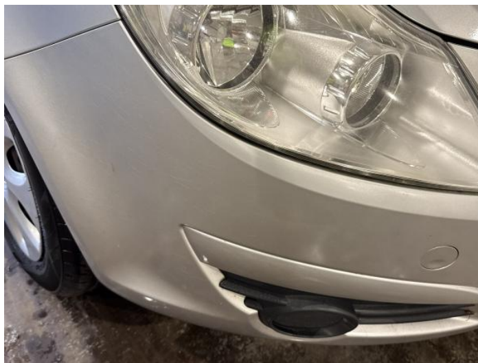
2: Bumper Front Scratched Over 100mm Thru Paint
