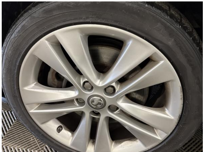
6: Wheel nsf Scratched Over 50mm
