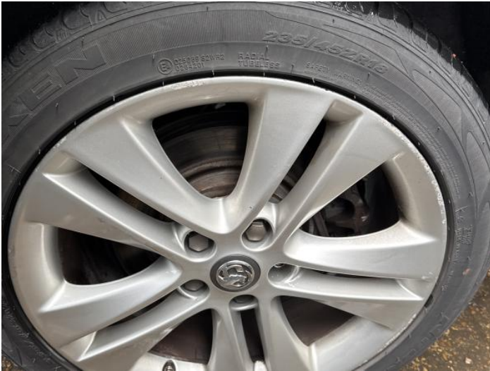
9: Wheel nsr Scratched Over 50mm
