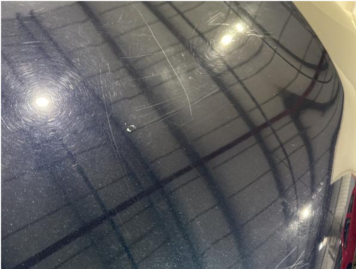
3: Bonnet Scratched Over 25mm Thru Paint
