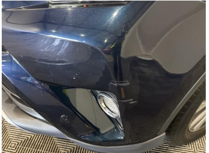
4: Bumper Front Scratched 25 to 100mm Thru Paint
