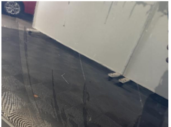
6: Door nsf Scratched Over 25mm Thru Paint
