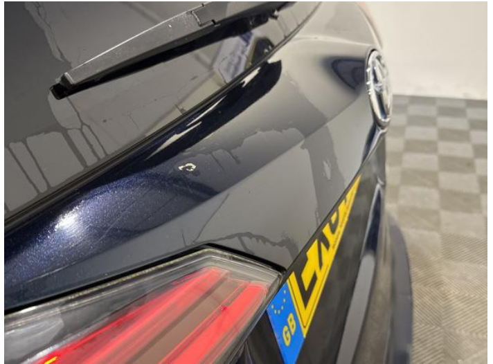
10: Tailgate Scratched Over 25mm Thru Paint
