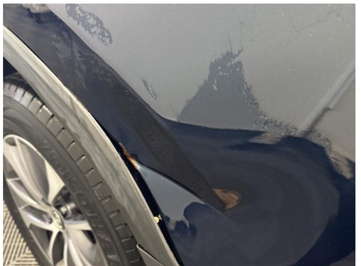
8: Qtr Panel nsr Dented With Paint Damage
