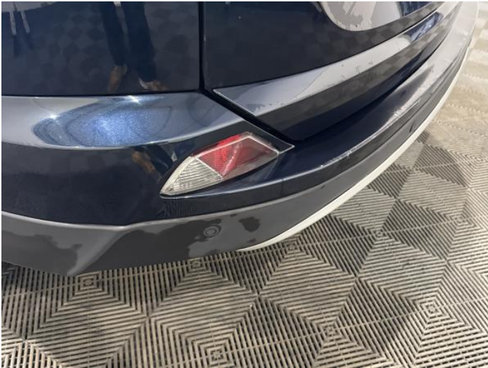
9: Bumper Rear Scratched Over 100mm Thru Paint
