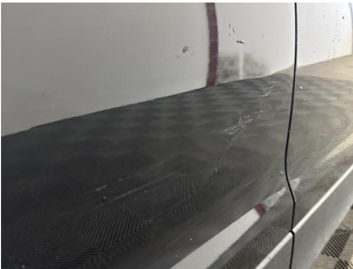
11: Door osr Dented With Paint Damage
