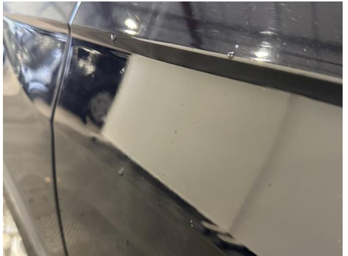
6: Door nsf Dented Between 10mm + 30mm
