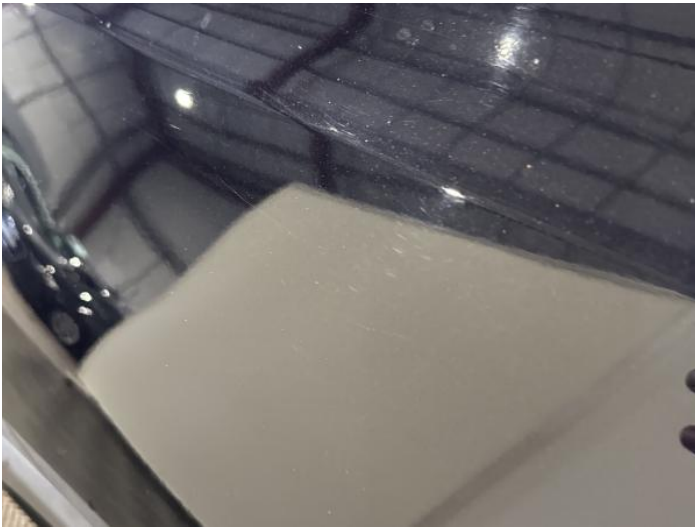
5: Wing nsf Scratched UpTo 25mm Thru Paint
