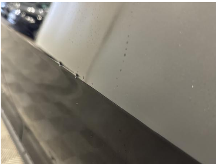
7: Door nsr Dented Between 10mm + 30mm
