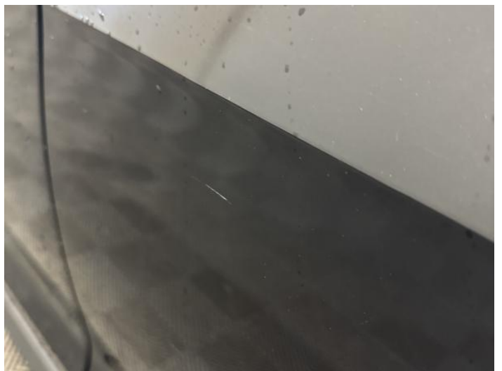
8: Door nsr Scratched UpTo 25mm Thru Paint
