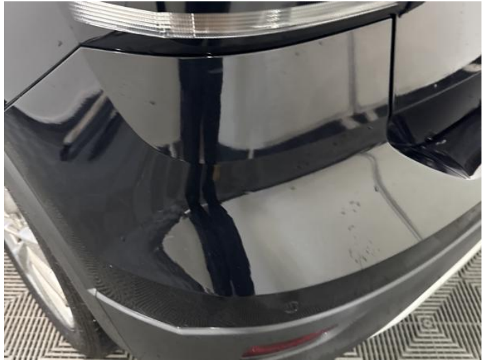
10: Bumper Rear Scratched 25 to 100mm Thru Paint
