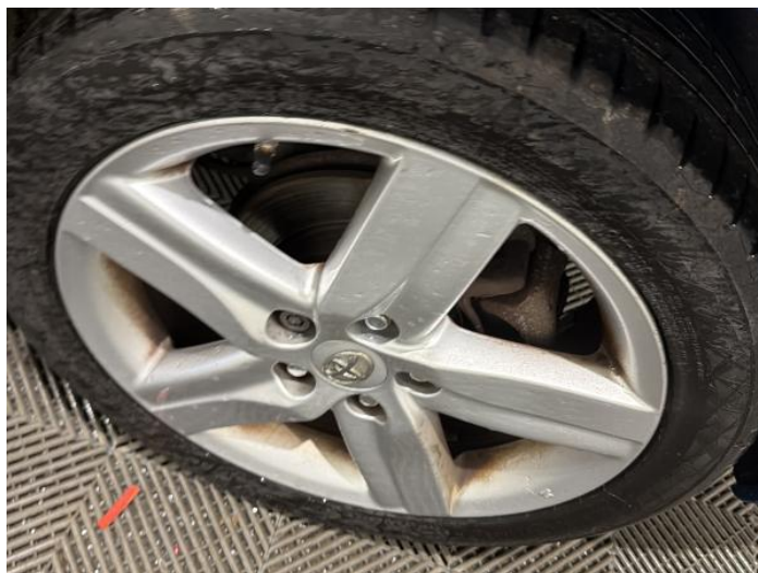
10: Wheel nsr Scratched Up To 50mm
