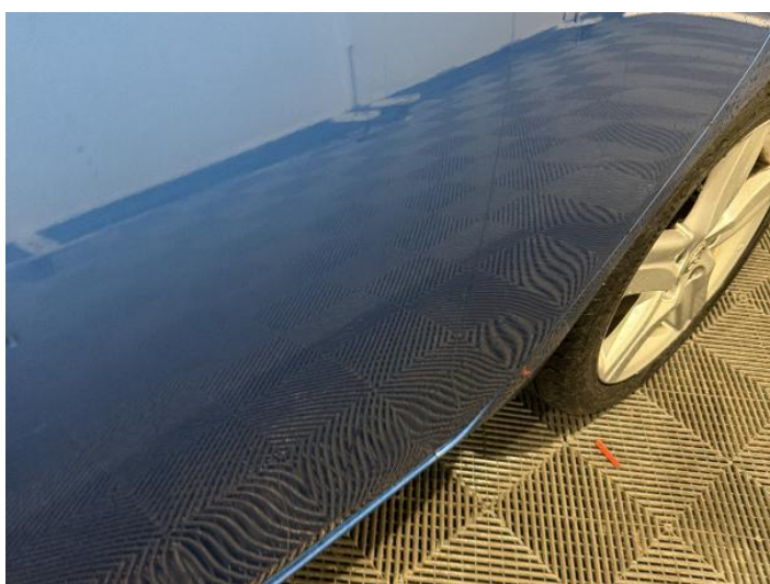
7: Door nsr Scratched UpTo 25mm Thru Paint
