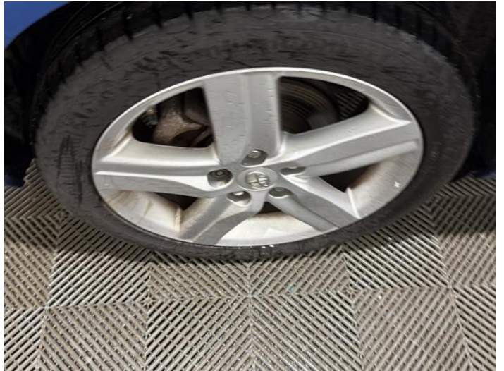
16: Wheel osr Scratched Up To 50mm
