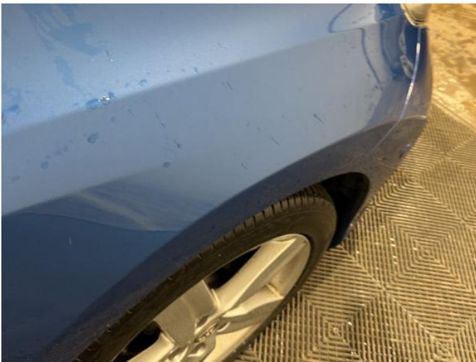
23: Wing osf Chipped 1 To 5
