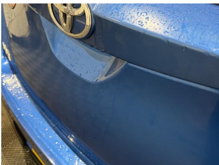
13: Boot Lid Dented Over 2 UpTo 10mm
