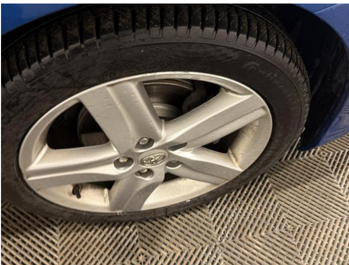
25: Wheel osf Scratched Over 50mm
