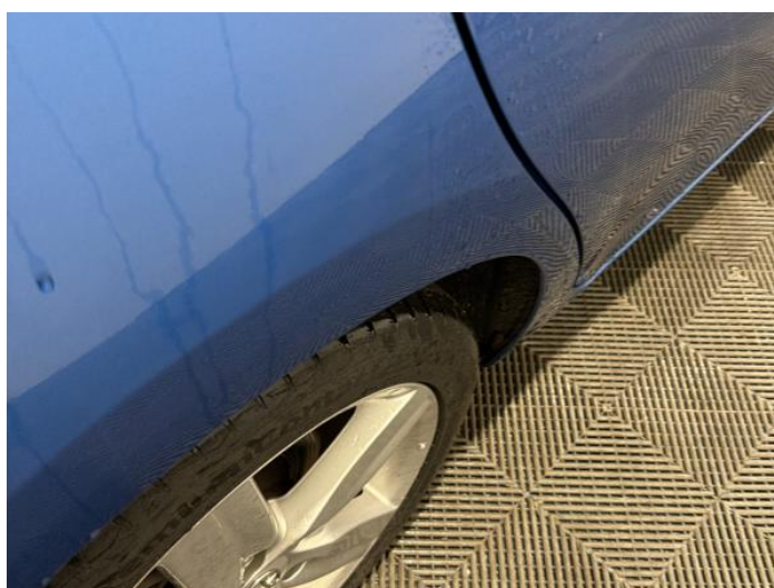
14: Qtr Panel osr Dented 2 Or Less UpTo 10mm
