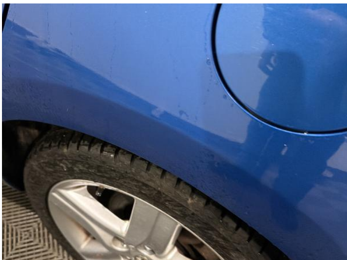
9: Qtr Panel nsr Dented With Paint Damage
