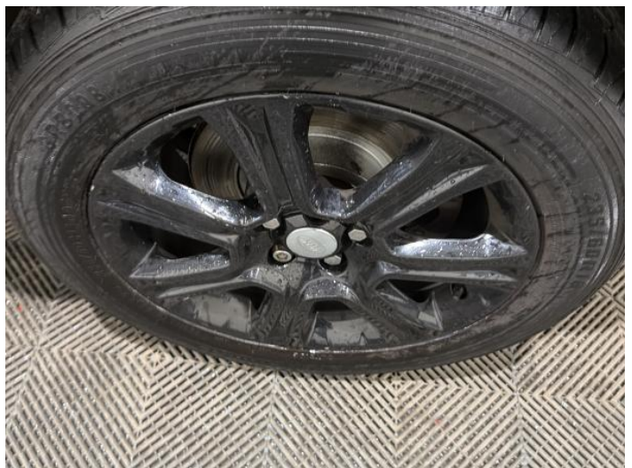
8: Wheel nsr Scratched Up To 50mm
