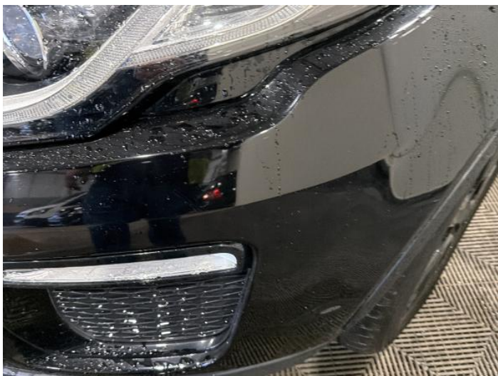
1: Bumper Front Chipped Multiple Chips
