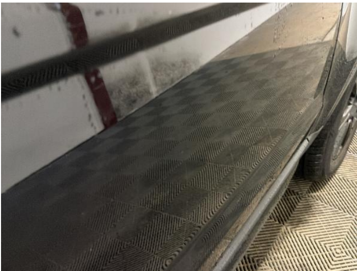
17: Door osf Dented Over 2 UpTo 10mm
