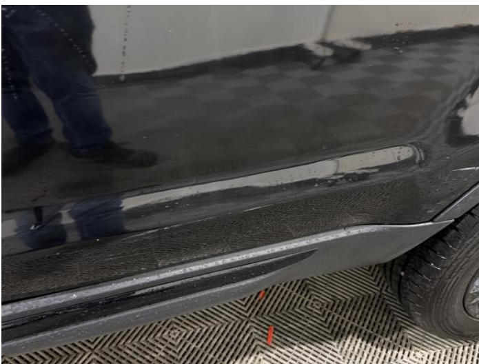
7: Door nsr Dented With Paint Damage
