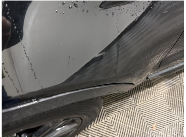
4: Wing nsf Poor Previous Repair Poor Paint
