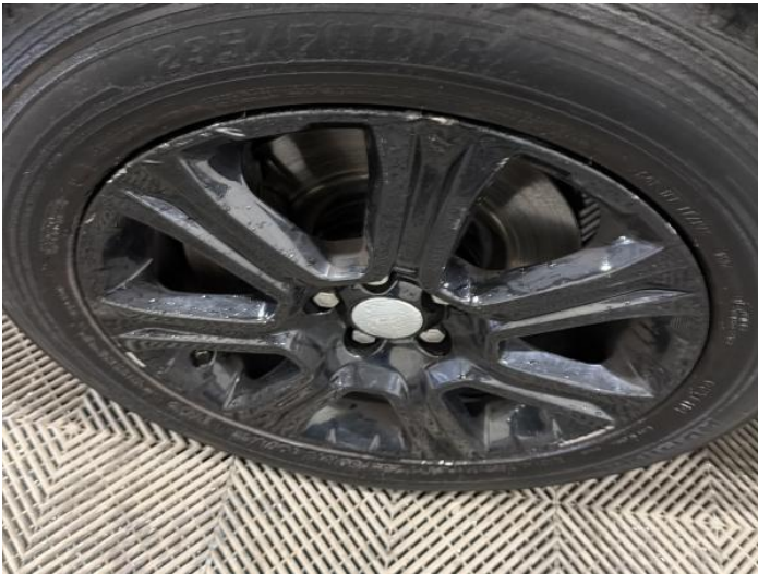
5: Wheel nsf Scratched Over 50mm
