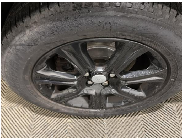
14: Wheel osr Scratched Up To 50mm
